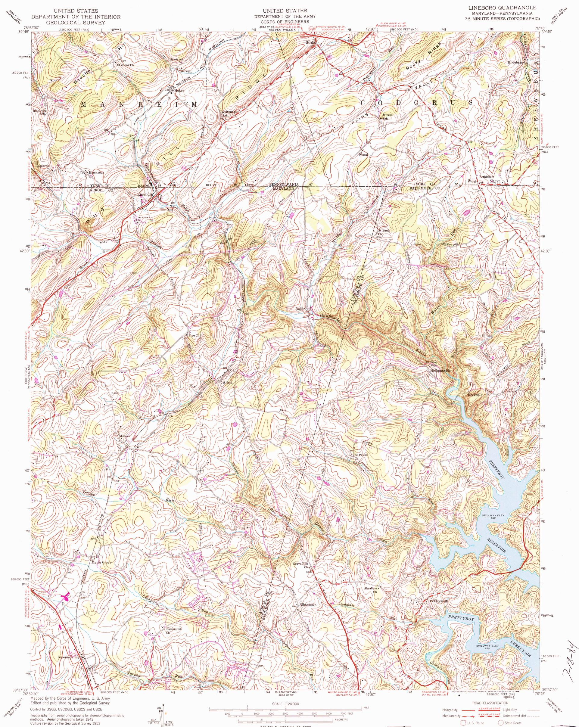
Polyconic projection. 1927 North American datum 10,000-foot grids based on Maryland coordinate system and Pennsylvania coordinate system, south zone 1000-metre Universal Transverse Mercator grid ticks, zone 18, shown in blue CONTOUR INTERVAL 20 FEET NATIONAL GEODETIC VERTICAL DATUM OF 1929
