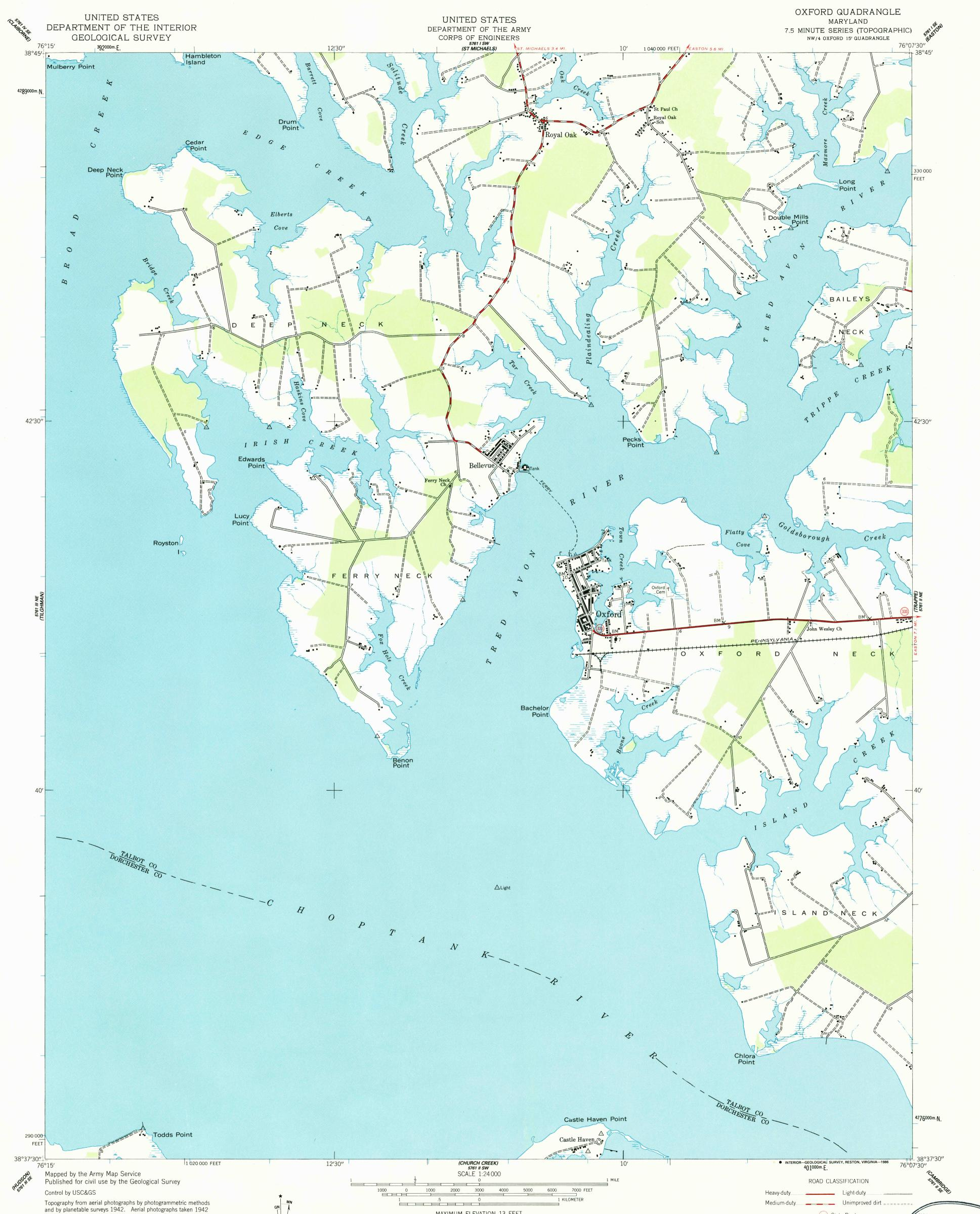
Polyconic projection. 1927 North American datum 10,000-foot grid based on Maryland coordinate system 1000-meter Universal Transverse Mercator grid ticks, zone 18, shown in blue
