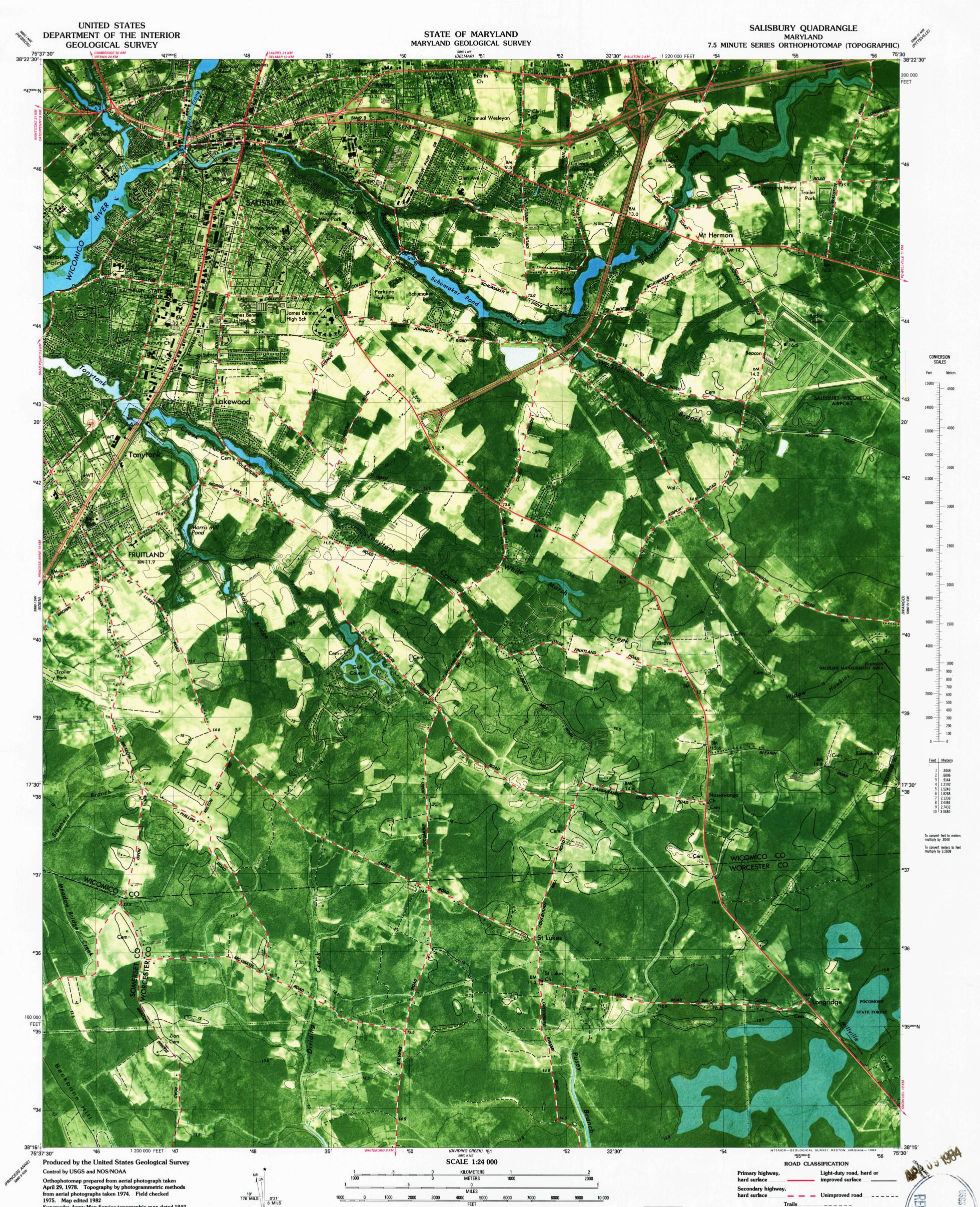
Supersedes Army Map Service topographic map dated 1942 Projection and 10,000-foot grid ticks: Maryland coordinate system (Lambert conformal conic) 1000-meter Universal Transverse Mercator grid, zone 18 1927 North American Datum To place on the predicted North American Datum 1983 move the projection lines 8 meters south and 31 meters west as shown by dashed corner ticks
