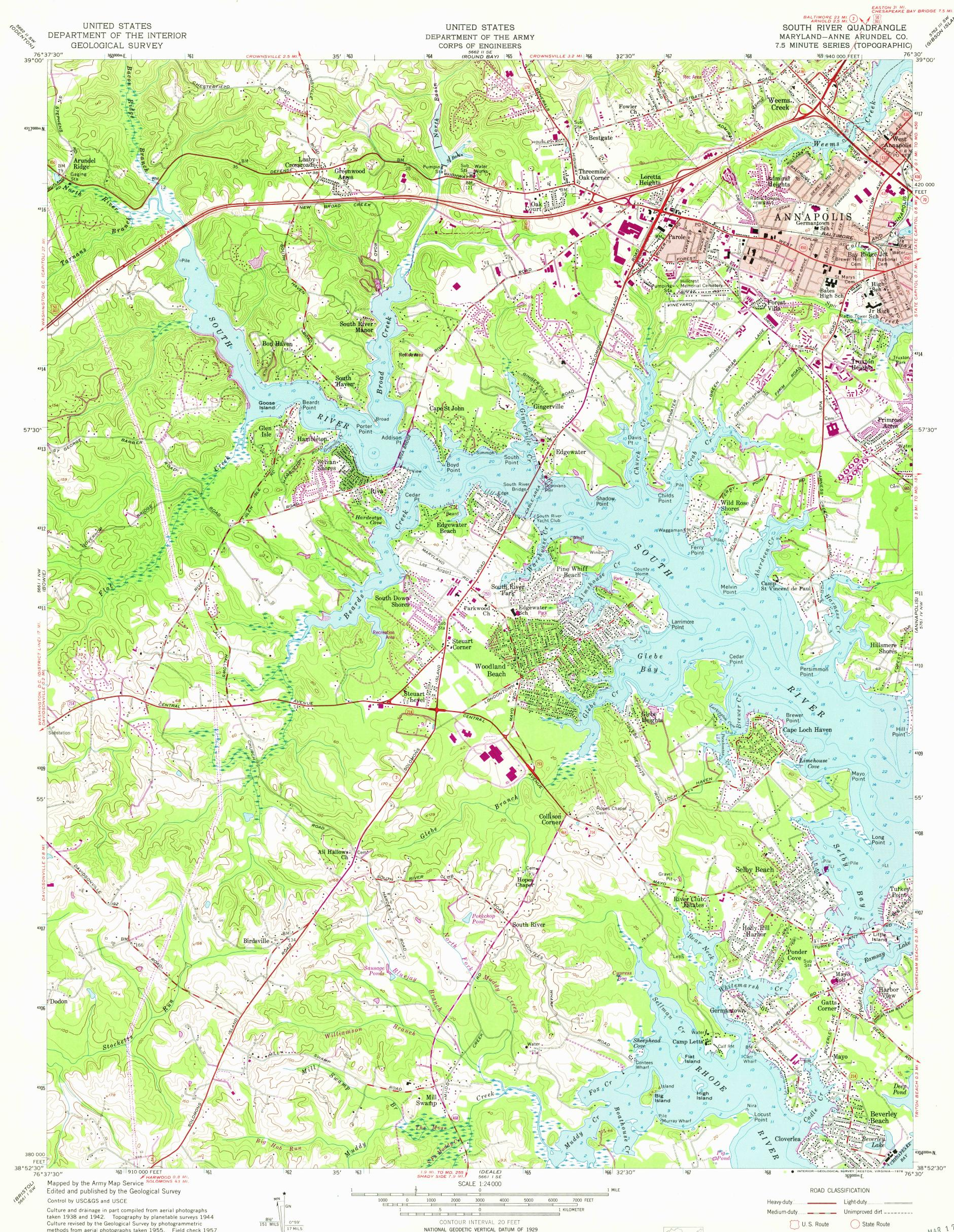
taken 1938 and 1942. Topography by planetable surveys 1944 Culture revised by the Geological Survey by photogrammetric methods from aerial photographs taken 1955. Field check 1957 Hydrography compiled from USC&GS chart 550 (1957)
