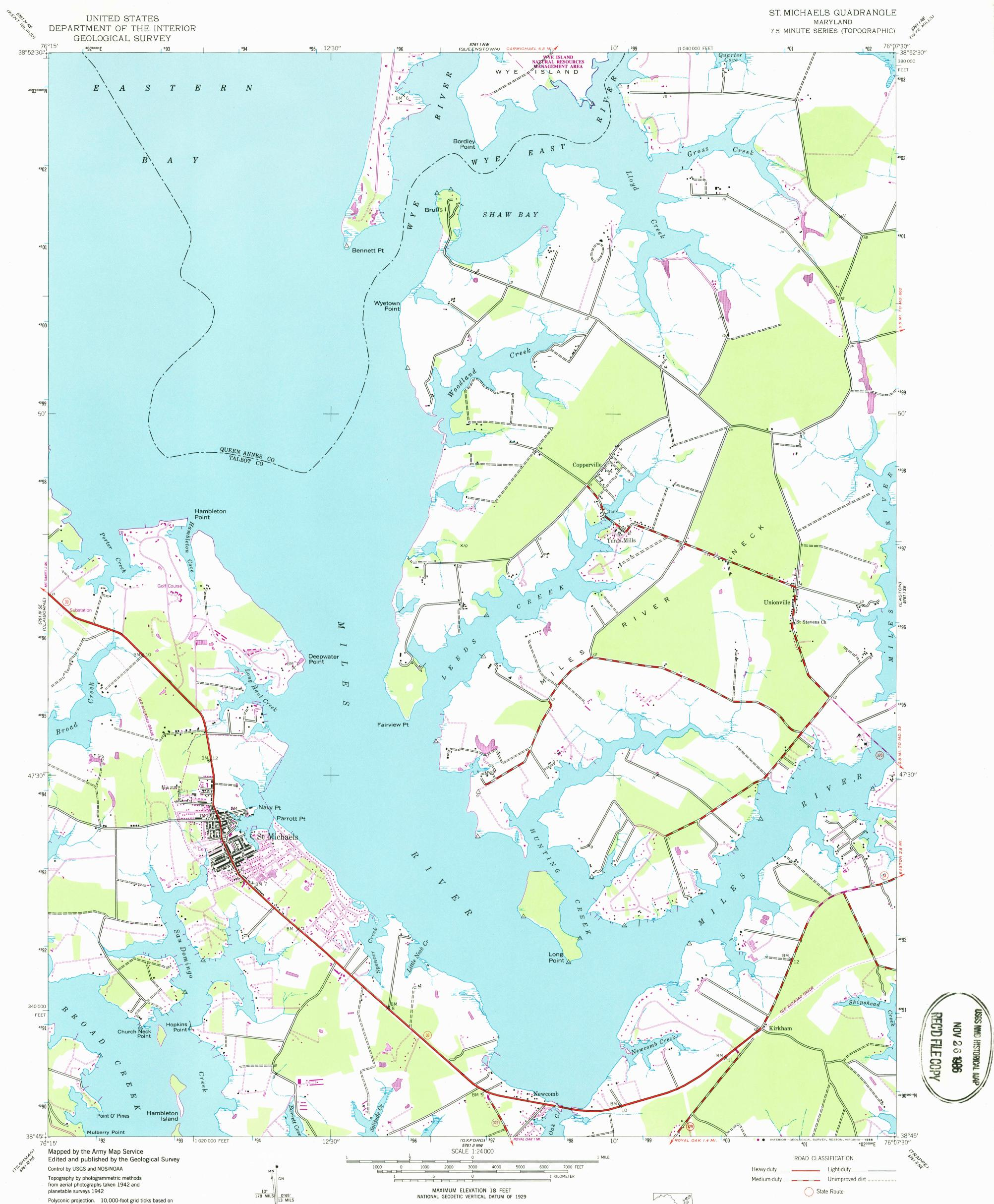
Polyconic projection. 10,000-foot grid ticks based on Maryland coordinate system 1000-meter Universal Transverse Mercator grid ticks, zone 18, shown in blue 1927 North American Datum To place on the predicted North American Datum 1983 move the projection lines 8 meters south and 29 meters west as shown by dashed corner ticks There may be private inholdings within the boundaries of
