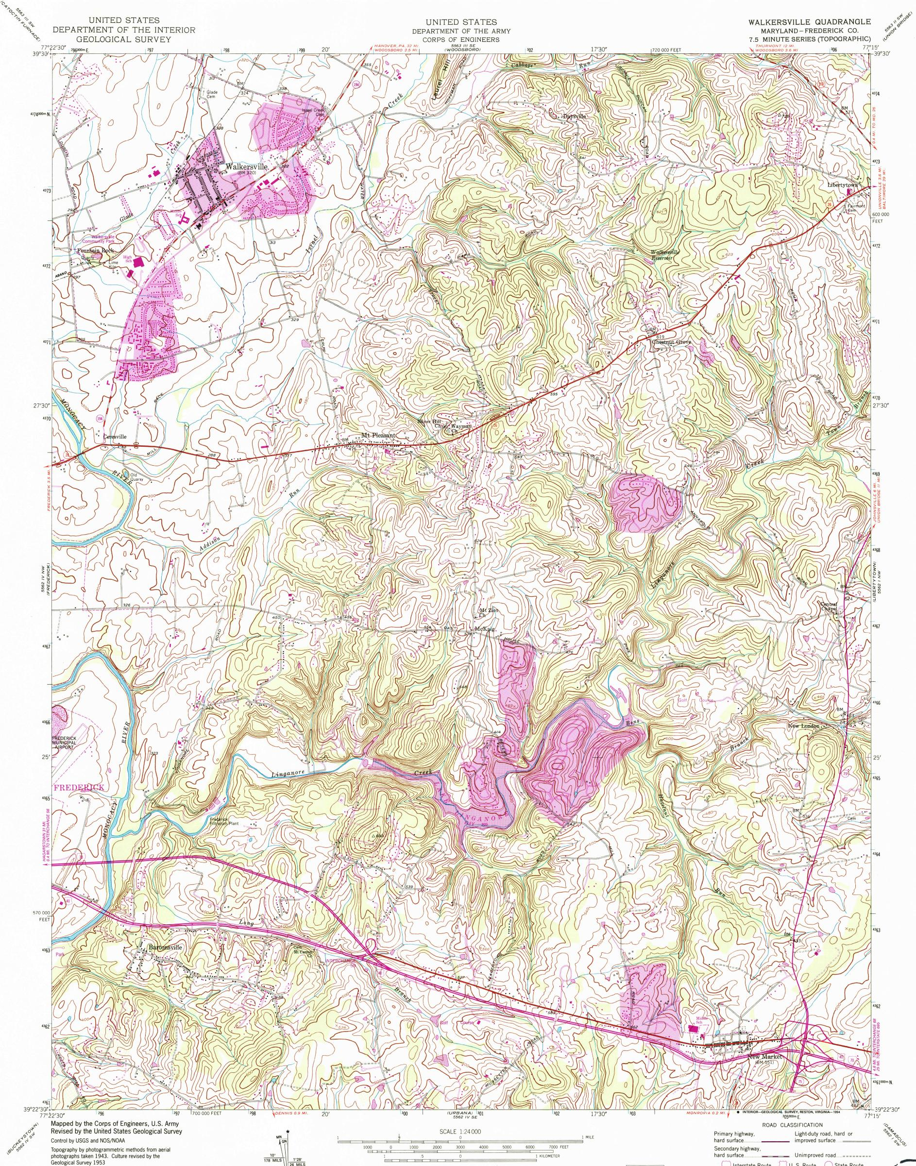
Projection and 10,000-foot grid ticks: Maryland coordinate system, (Lambert conformal conic) 1000-meter Universal Transverse Mercator grid ticks, zone 18, shown in blue 1927 North American Datum (NAD 27)
