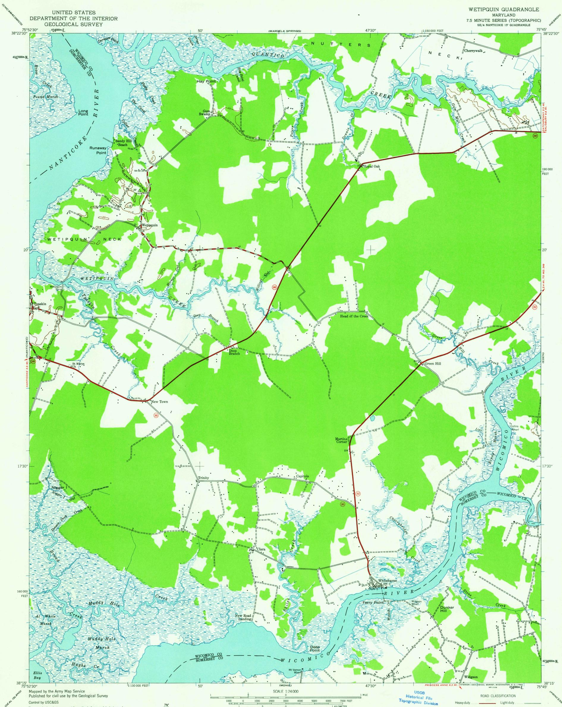
Topography by photogrammetric methods from aerial photographs taken 1942 and planetable surveys 1942
