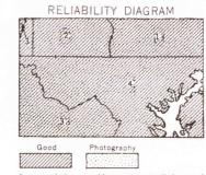
Large scale topographic maps, controlled ground survey, 1908-49. Planimetry revised from: 1-1947; 2-1949; 3-1950-51; 4-1952-53 aerial photography. BALTIMORE, MD., PA.; VA.; W. VA. 1957 REVISED 1969
