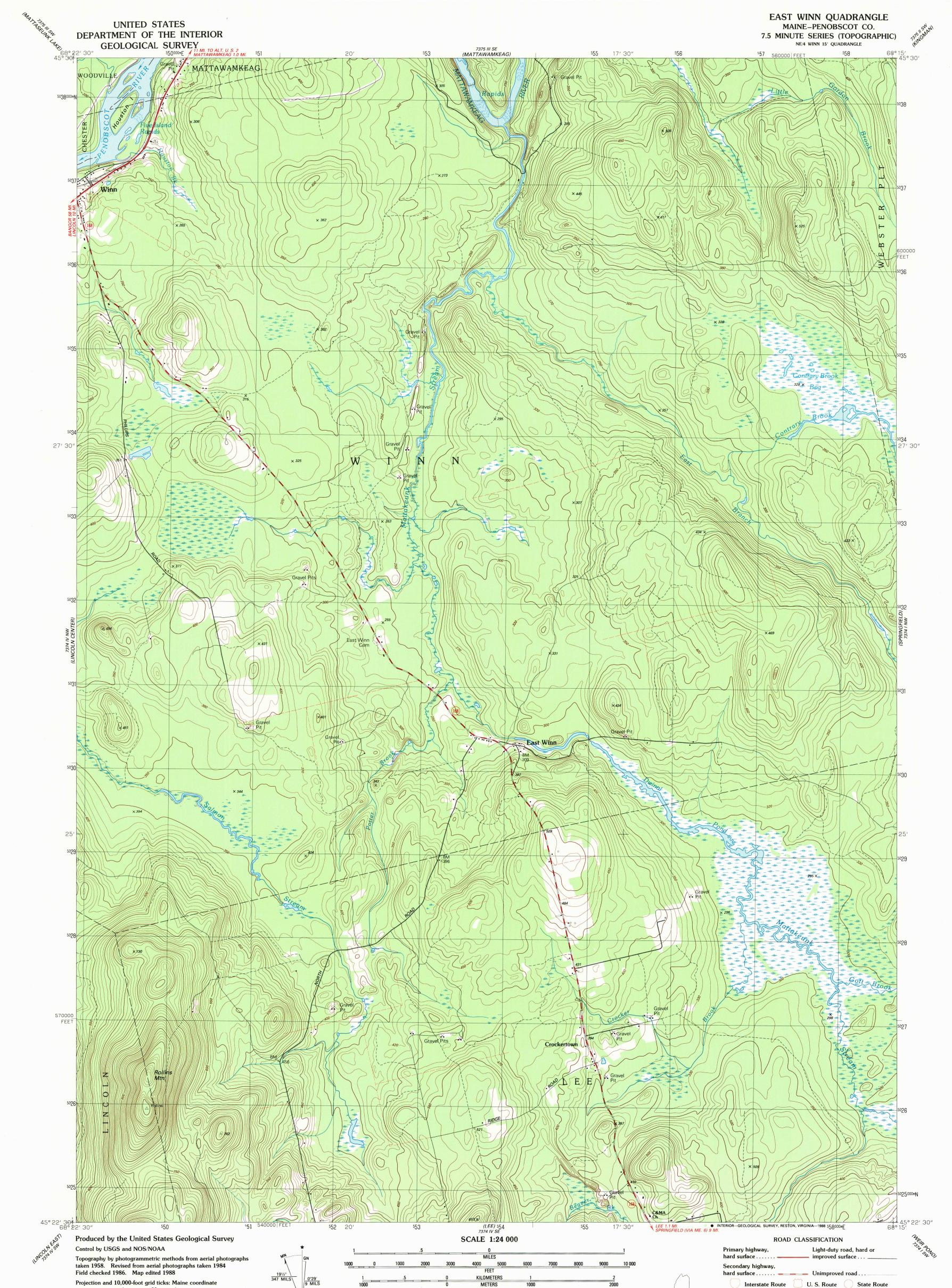
Projection and 10,000-foot grid ticks: Maine coordinate system, east zone (transverse Mercator) 1000-meter Universal Transverse Mercator grid, zone 19 1927 North American Datum To place on the predicted North American Datum 1983, move the projection lines 1 meter south and 45 meters west as shown by dashed corner ticks
