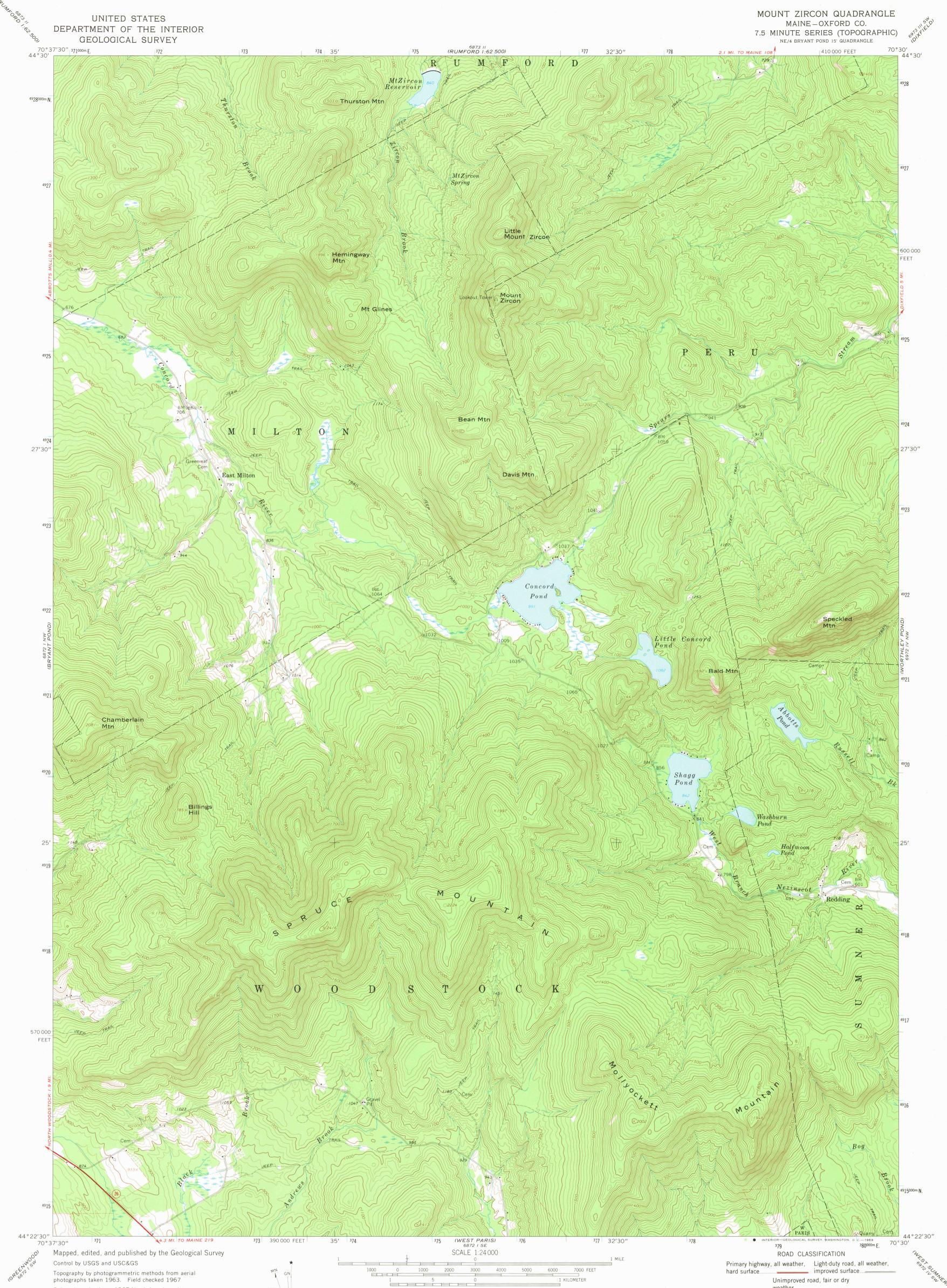
Polyconic projection. 1927 North American datum 10,000-foot grid based on Maine coordinate system, west zone 1000-meter Universal Transverse Mercator grid ticks, zone 19, shown in blue
