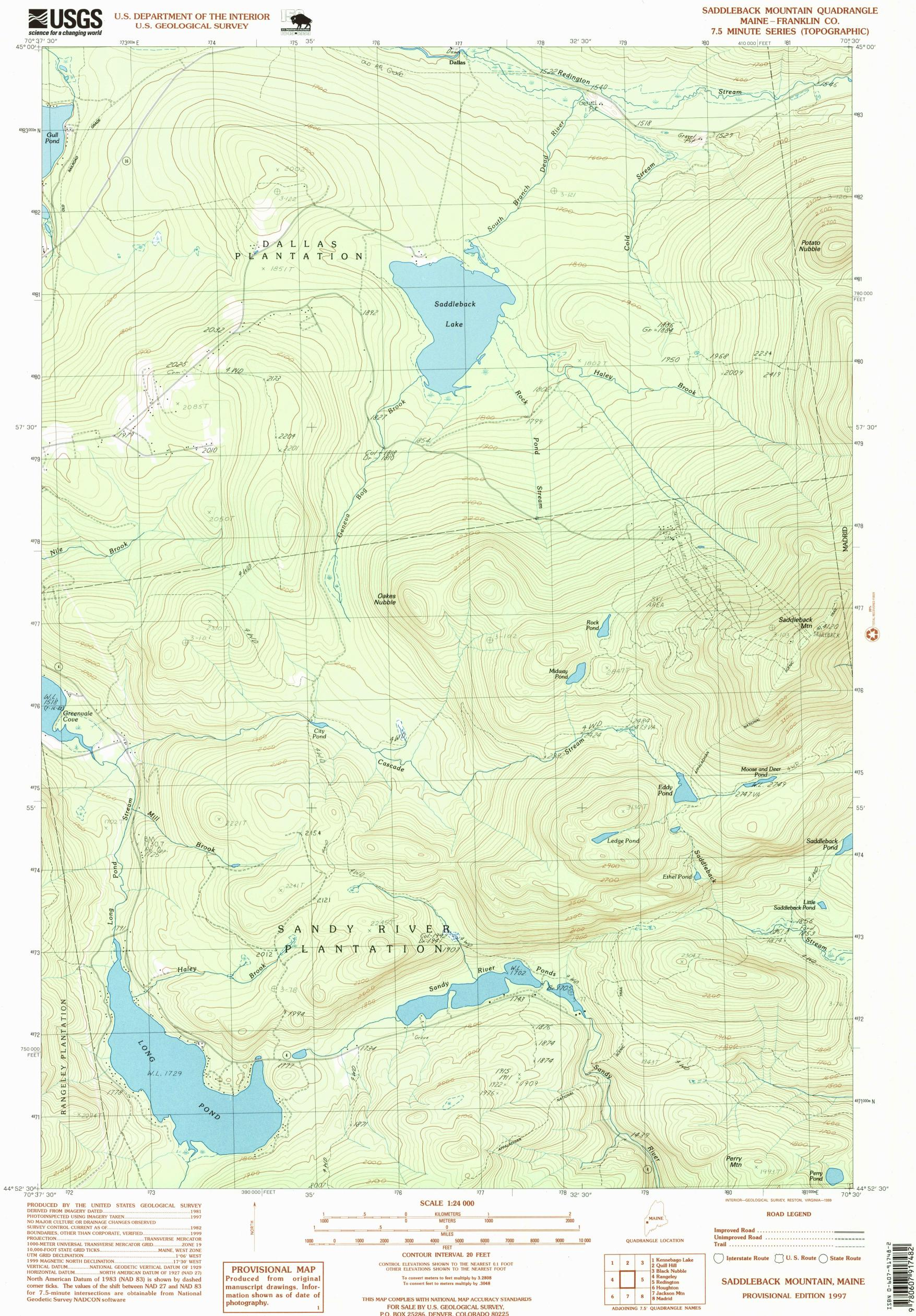
.....ZONE 19 10,000-FOOT STATE GRID TICKS..... ......MAINE, WEST ZONE North American Datum of 1983 (NAD 83) is shown by dashed corner ticks. The values of the shift between NAD 27 and NAD 83 for 7.5-minute intersections are obtainable from National Geodetic Survey NADCON software
