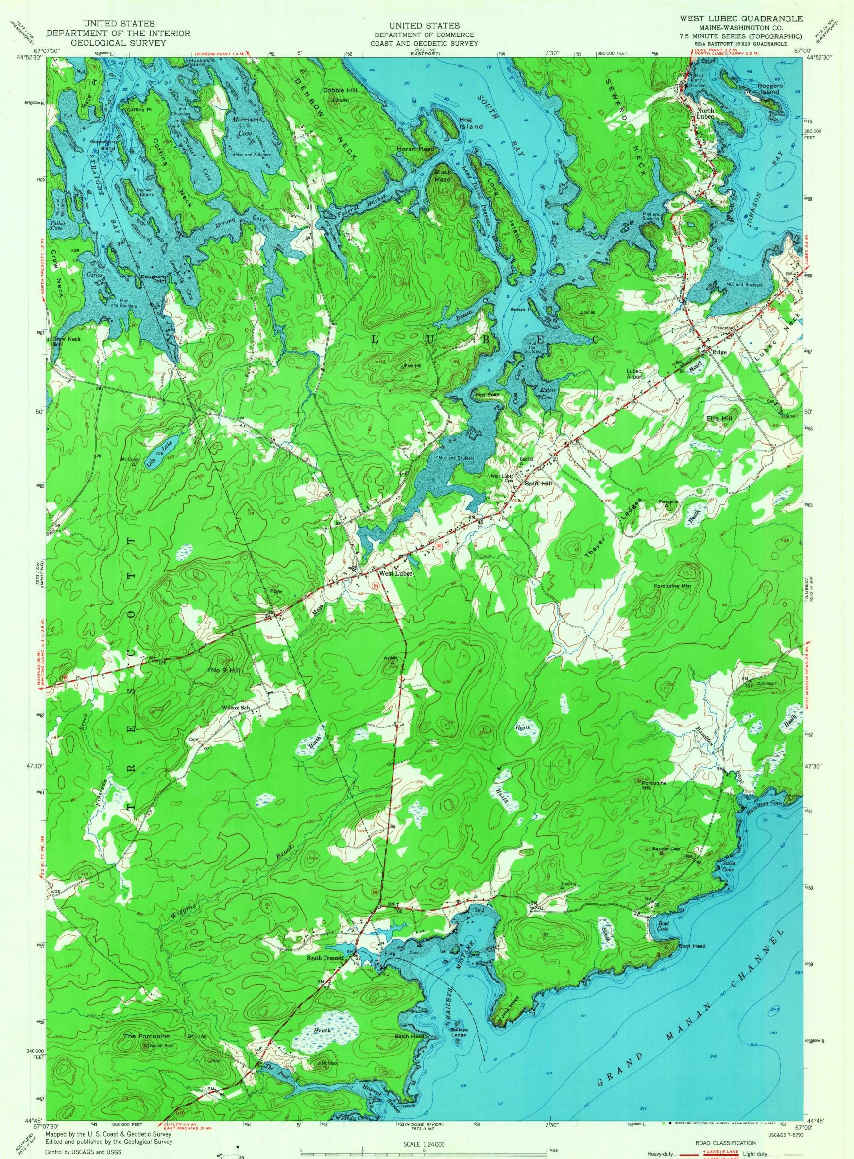
Topography from aerial photographs by multiplex methods Aerial photographs taken 1946. Field check 1949 Hydrography from surveys dated 1866-1890 Polyconic projection. 1927 North American datum 10,000-foot grid based on Maine coordinate system, east zone UTM GRID AND 1949 MAGNETIC NORTH DECLINATION AT CENTER OF SHEET Unchecked elevations are shown in brown 1000-meter Universal Transverse Mercator grid ticks,
