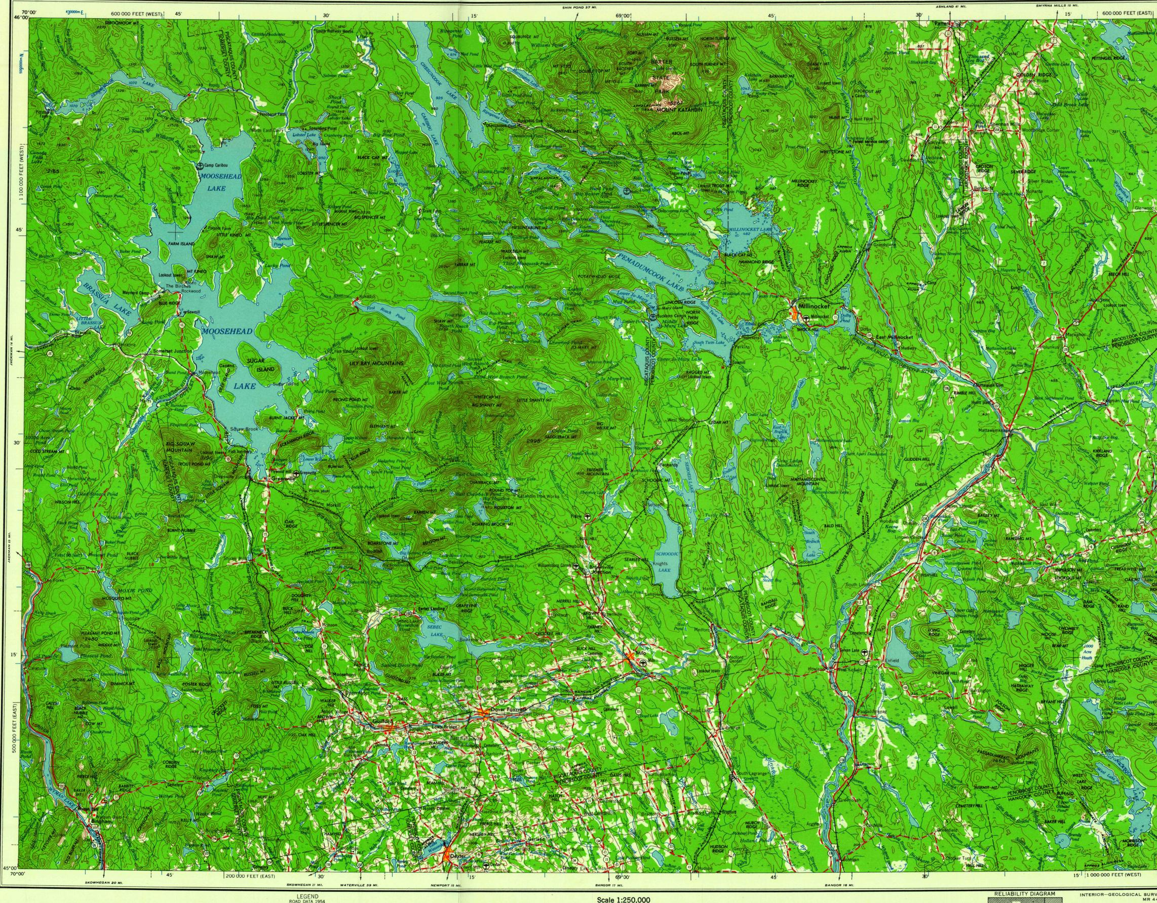
Prepared by the Army Map Service (AMGN), Corps of Engineers, U. S. Army, Washington, D. C. Compiled in 1954 by photogrammetric methods and from: United States Quadrangles, 1.50,000, 1:62,500, Corps of Engineers, and U. S. Geological Survey, 1903-49. Planimetric detail revised by photoplani-metric methods. Horizontal and vertical control by USC&GS and USGS. Map field checked 1954 100,000-foot grids based on Maine coordinate system, east and west zones
