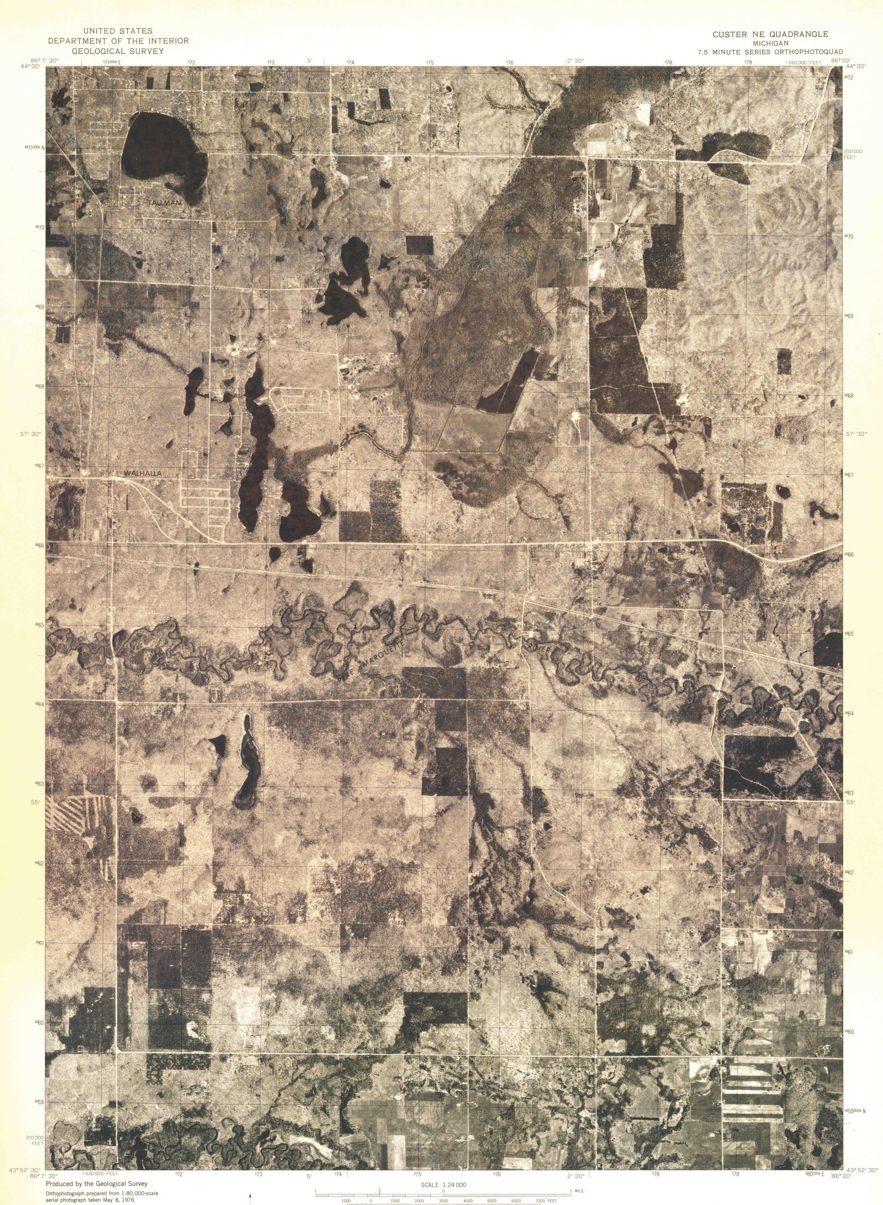
Projection and 10,000-foot grid ticks: Michigan coordinate system, central zone (Lambert conformal conic) 1000-meter Universal Transverse Mercator grid, zone 16. 1927 North American datum
