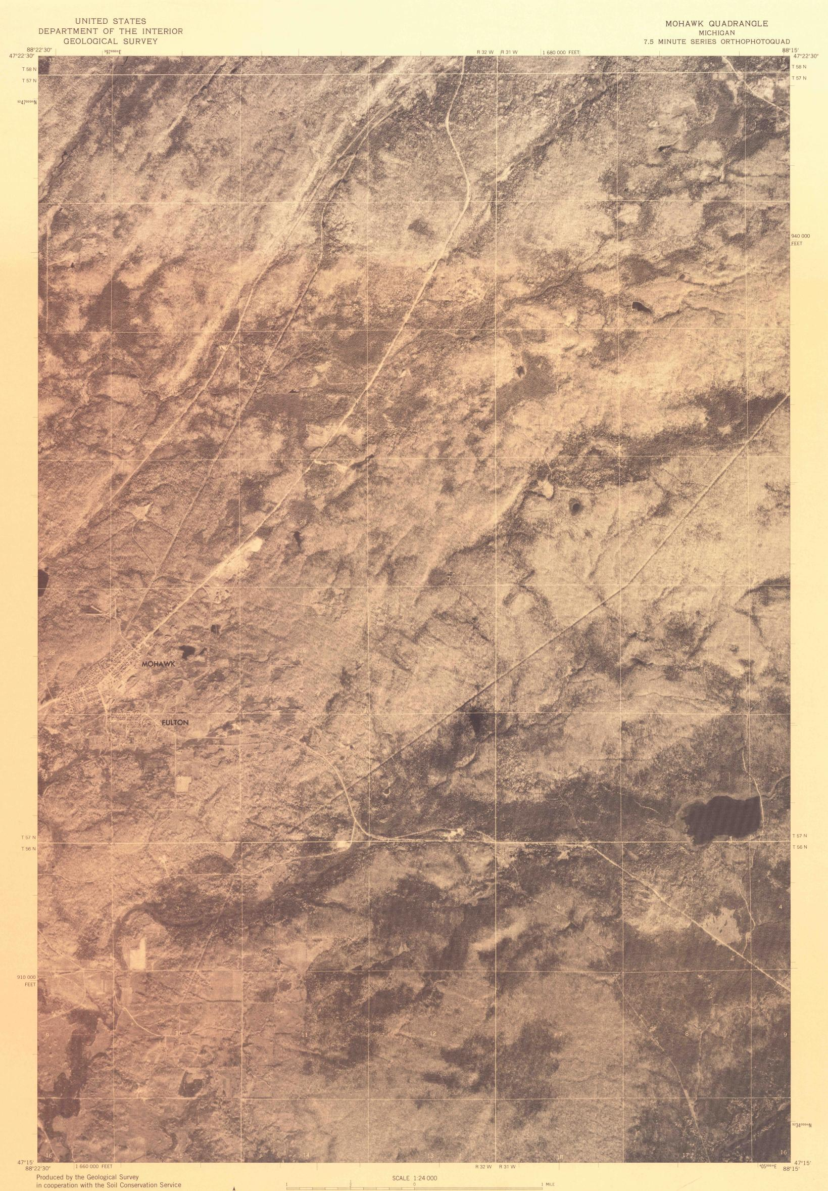
Projection and 10,000-foot grid ticks: Michigan coordinate system, north zone (Lambert conformal conic) 1000-meter Universal Transverse Mercator grid ticks, zone 16. 1927 North American Datum
