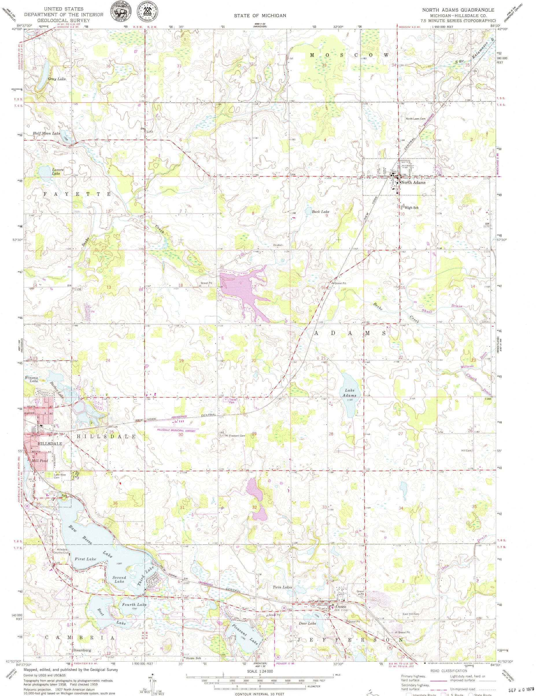
10,000-foot grid based on Michigan coordinate system, south zone To place on the predicted North American Datum 1983 move the proejction lines 0 meters north and 3 meters west as shown by dashed corner ticks 1000-meter Universal Transverse Mercator grid ticks, zone 16, shown in blue Red tint indicates areas in which only landmark buildings are shown
