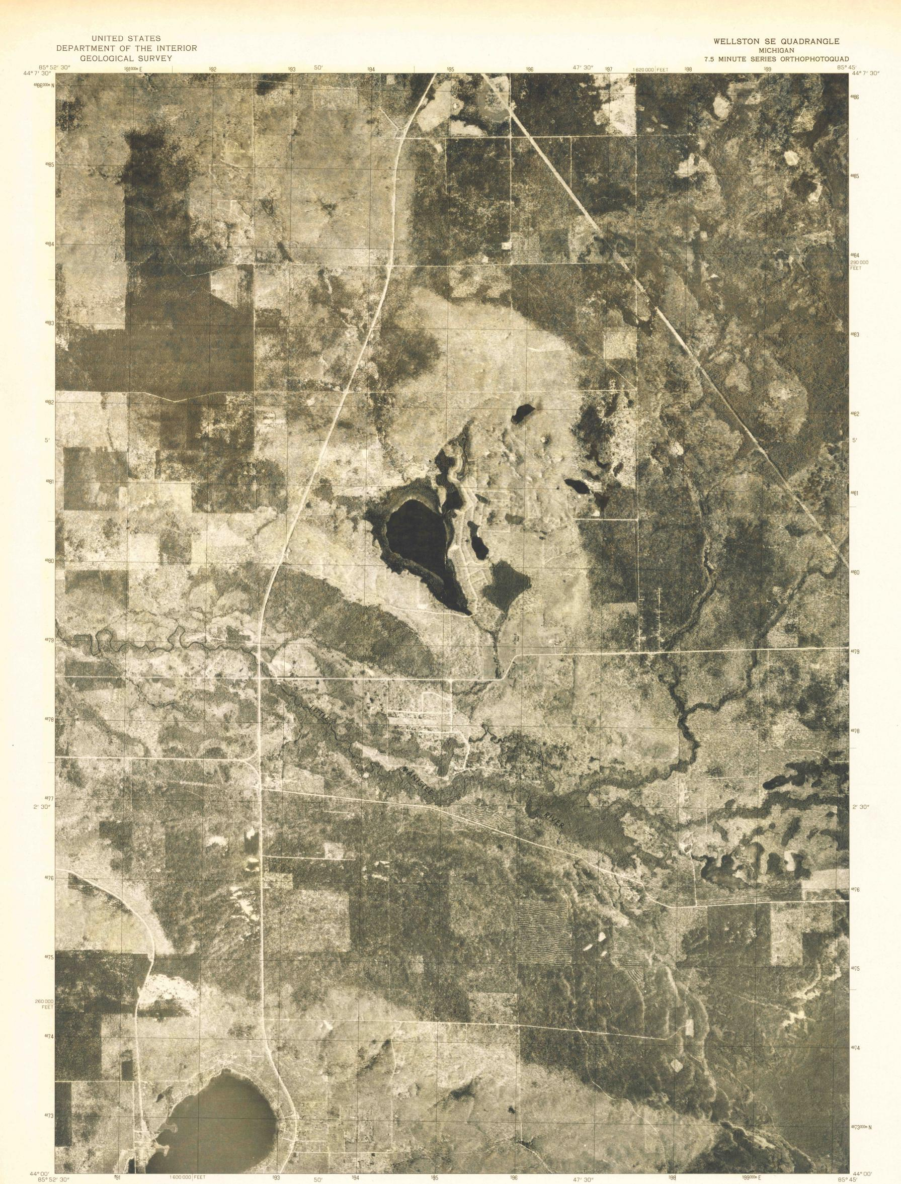
Produced by the Geological Survey Orthophotograph prepared from 1:80,000-scale aerial photograph taken May 8, 1976 Projection and 10,000-foot grid ticks: Michigan coordinate system, central zone (Lambert conformal conic) 1000-meter Universal Transverse Mercator grid, zone 16. 1927 North American datum
