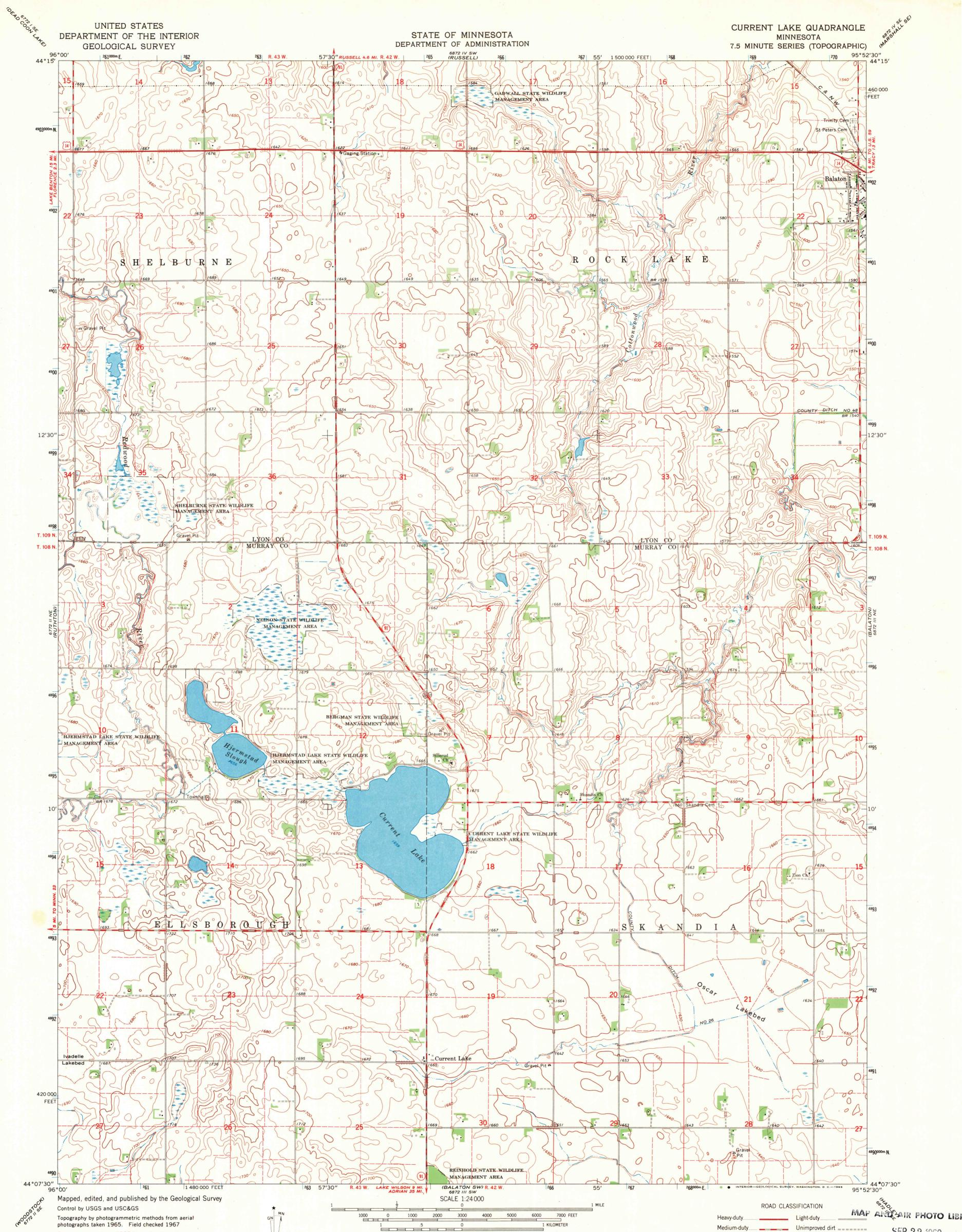
Polyconic projection. 1927 North American datum 2°03' 36 MILS 10,000-foot grid based on Minnesota coordinate system, south zone 1000-meter Universal Transverse Mercator grid ticks, zone 15, shown in blue
