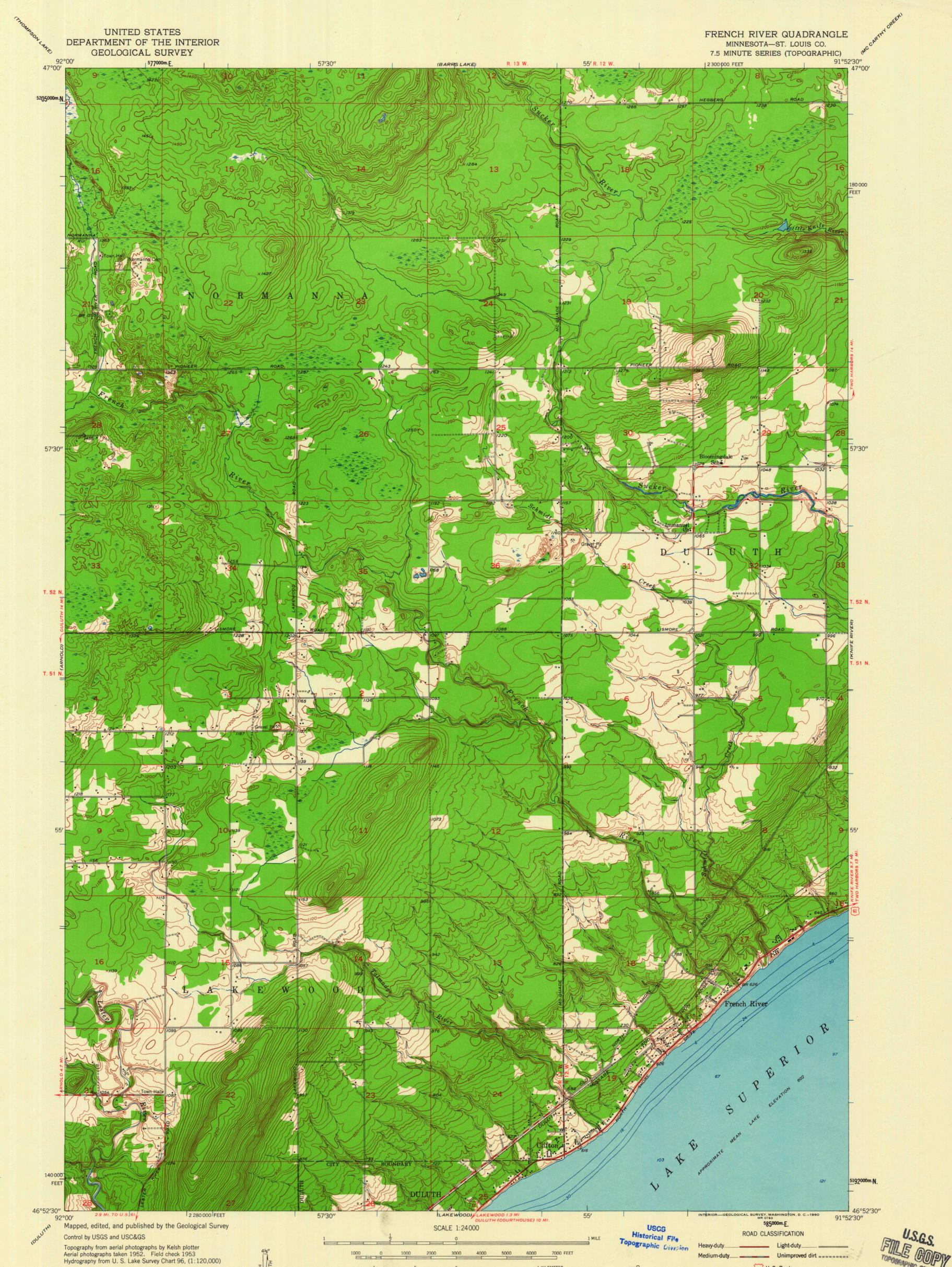
Topography from aerial photographs by Kelsh plotter Aerial photographs taken 1952. Field check 1953 Hydrography from U. S. Lake Survey Chart 96, (1:120,000) Polyconic projection. 1927 North American datum 10,000-foot grid based on Minnesota coordinate system, north zone
