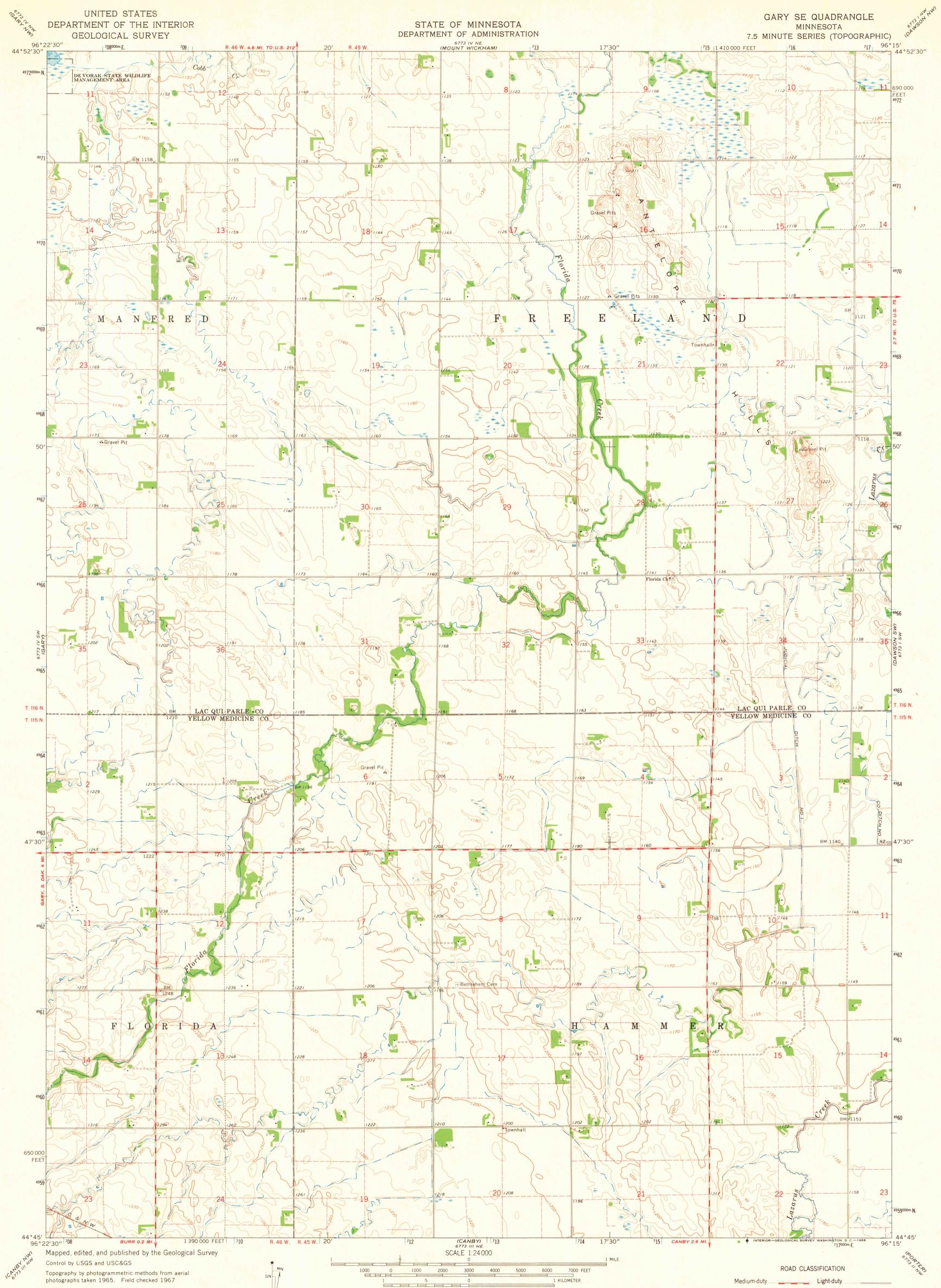
Polyconic projection. 1927 North American datum 10,000-foot grid based on Minnesota coordinate system, south zone 1000-meter Universal Transverse Mercator grid ticks, zone 14, shown in blue
