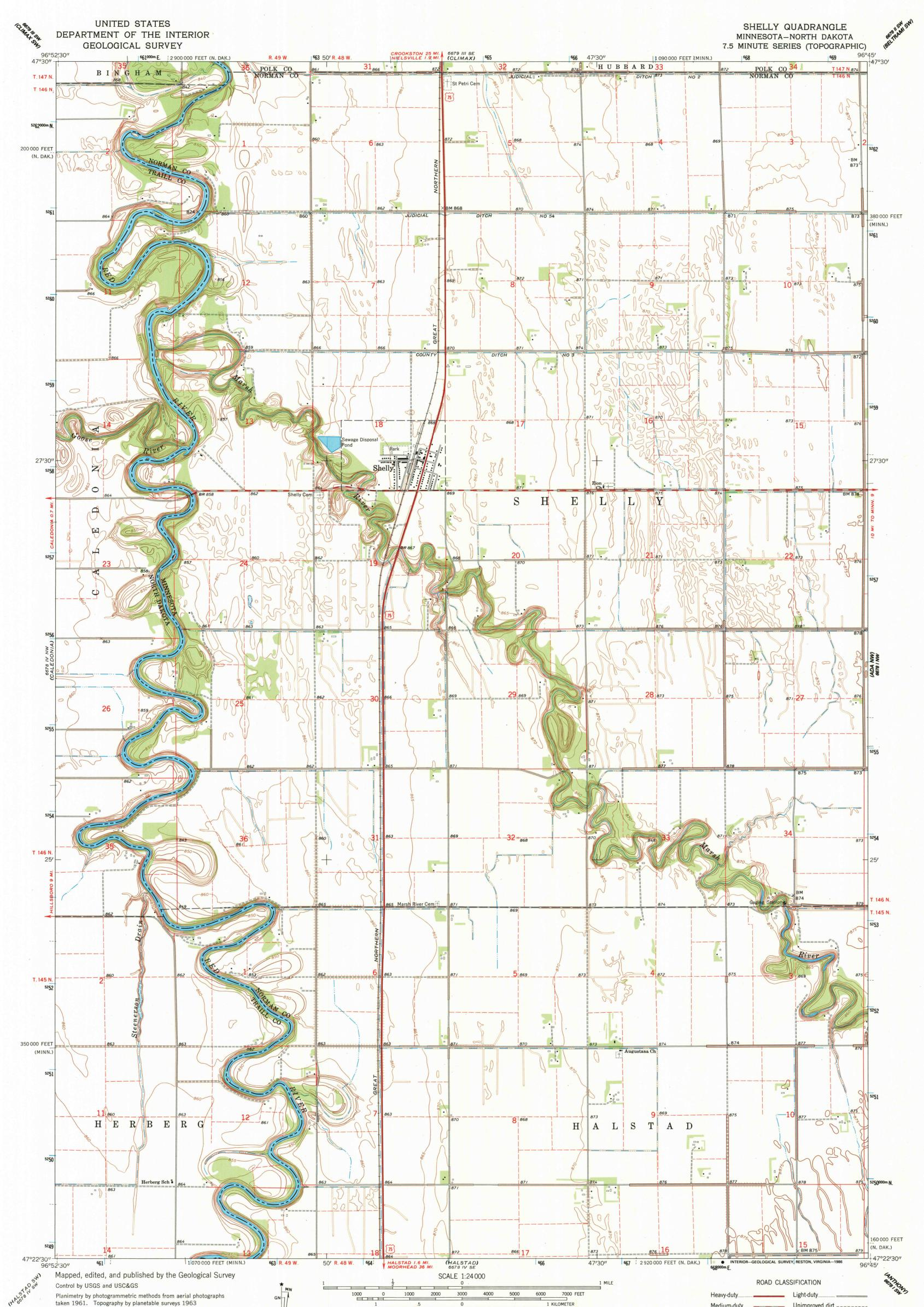
Planimetry by photogrammetric methods from aerial photographs taken 1961. Topography by planetable surveys 1963
