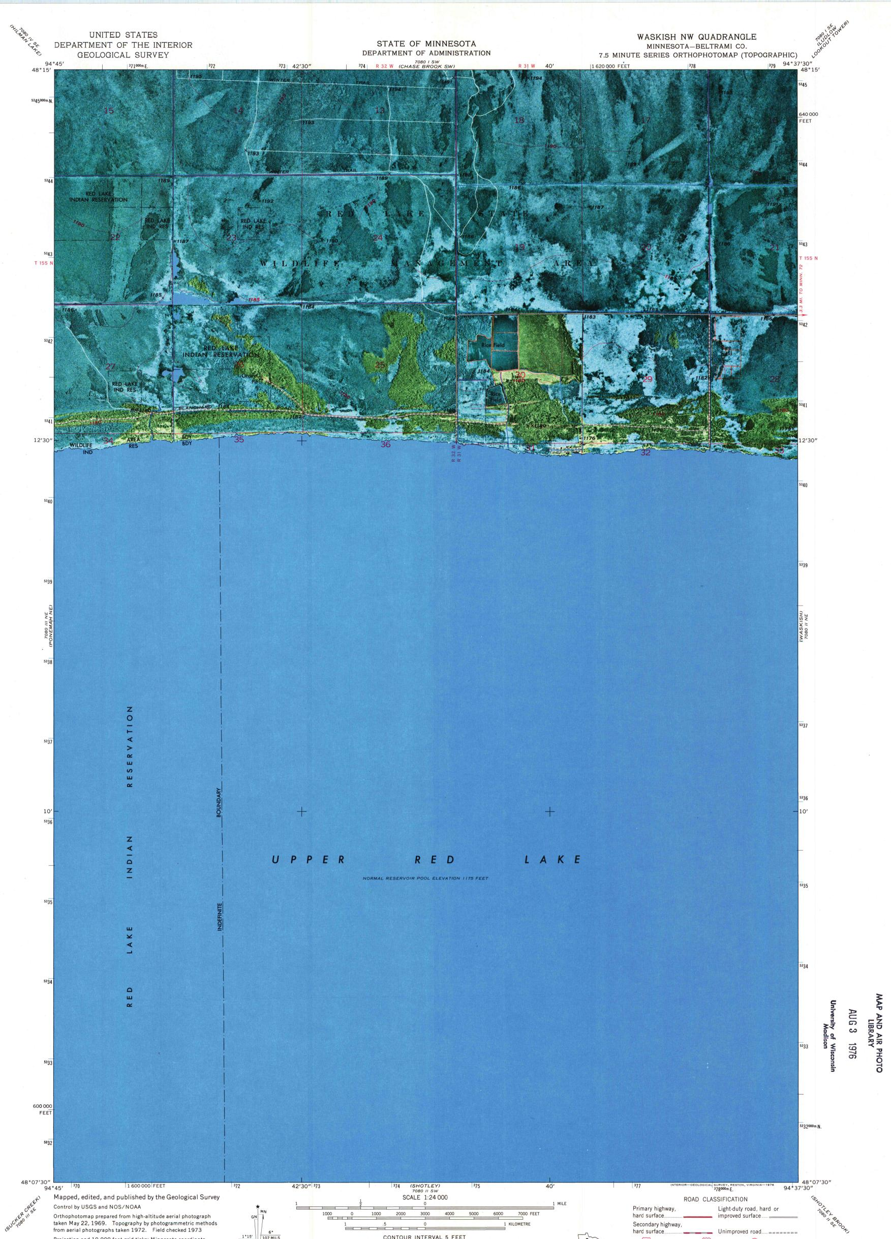
Orthophotomap prepared from high-altitude aerial photograph taken May 22, 1969. Topography by photogrammetric methods from aerial photographs taken 1972. Field checked 1973
