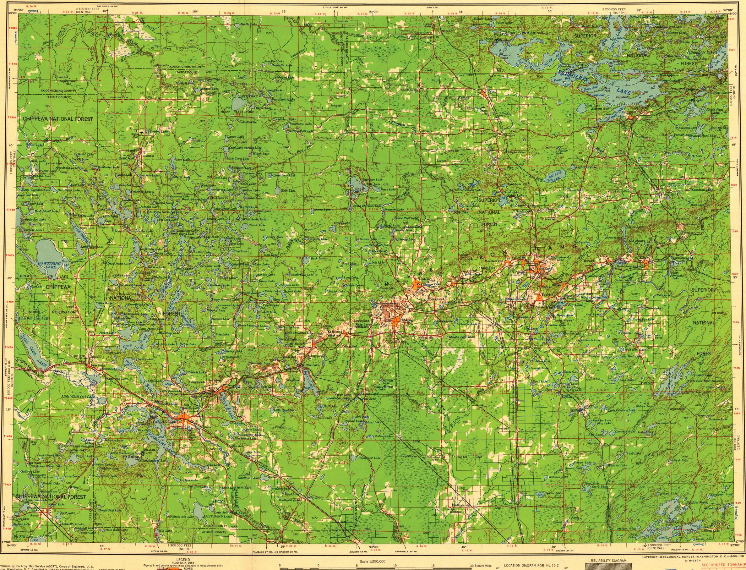
Prepared by the Army Map Service (ASCTT), Corps of Engineers, U. S. Army, Washington, D. C. Compiled in 1955 by photogrammetric methods and from: Minnesota, 1:20,000 and 1:24,000 USGS, 1949-1953. Planimetric detail revised by photo-planimetric methods. Horizontal and vertical control by USC&GS, USGS, and USFS. Photography field annotated 1954. 100,000-foot grids based on Minnesota coordinate system,
