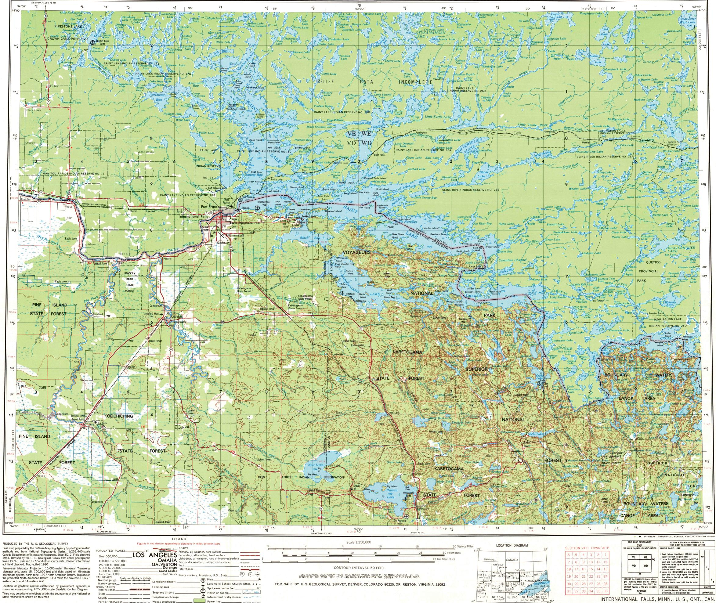
coordinate system, north zone. 1927 North American Datum. To place on the predicted North American Datum 1983 move the projection lines 5 meters north and 14 meters east
