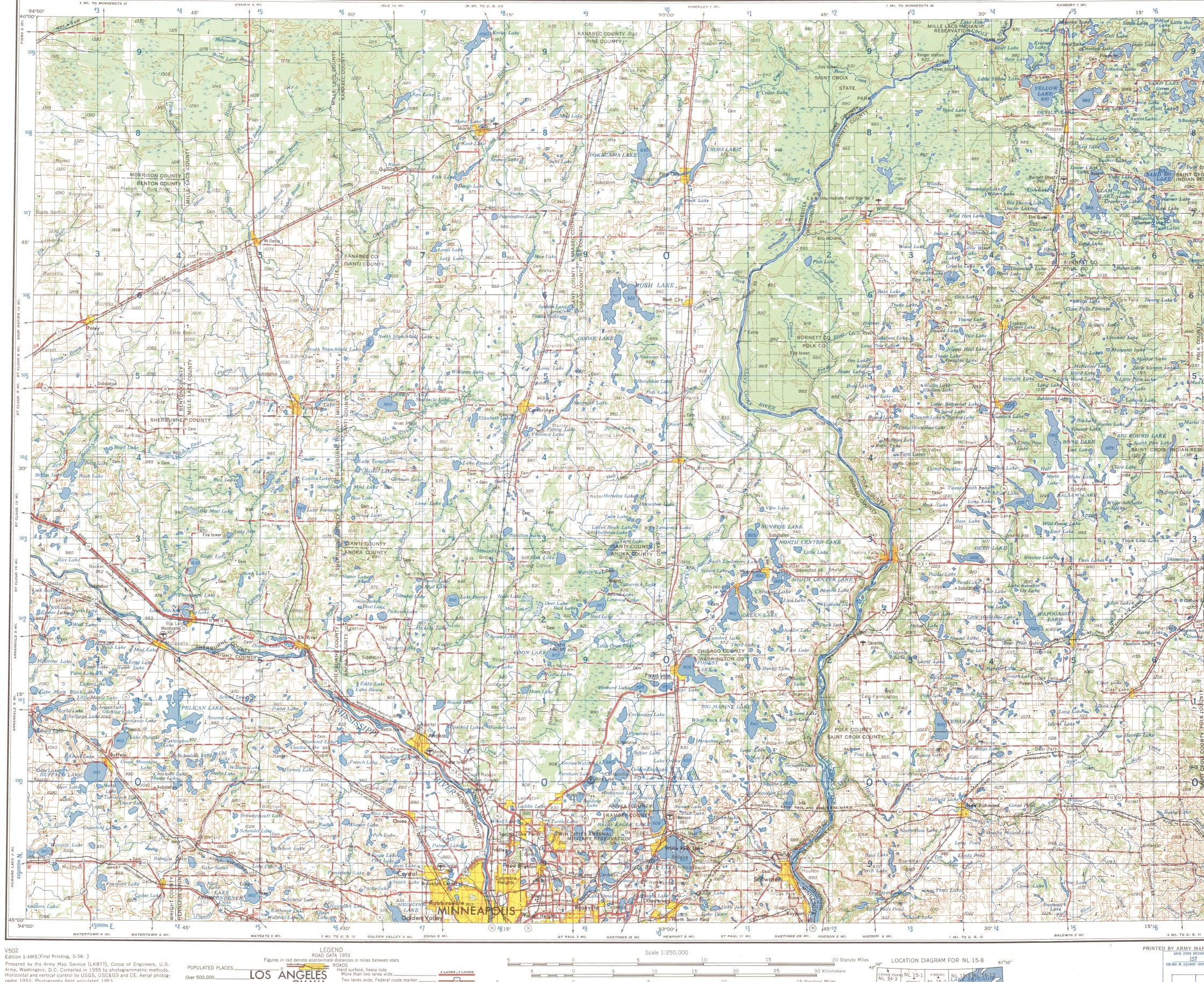
Prepared by the Army Map Service (LKBTT), Corps of Engineers, U.S. Army, Washington, D.C. Compiled in 1955 by photogrammetric methods. Horizontal and vertical control by USGS, USC&GS and CE. Aerial photog-raphy 1953. Photography field annotated 1953.
