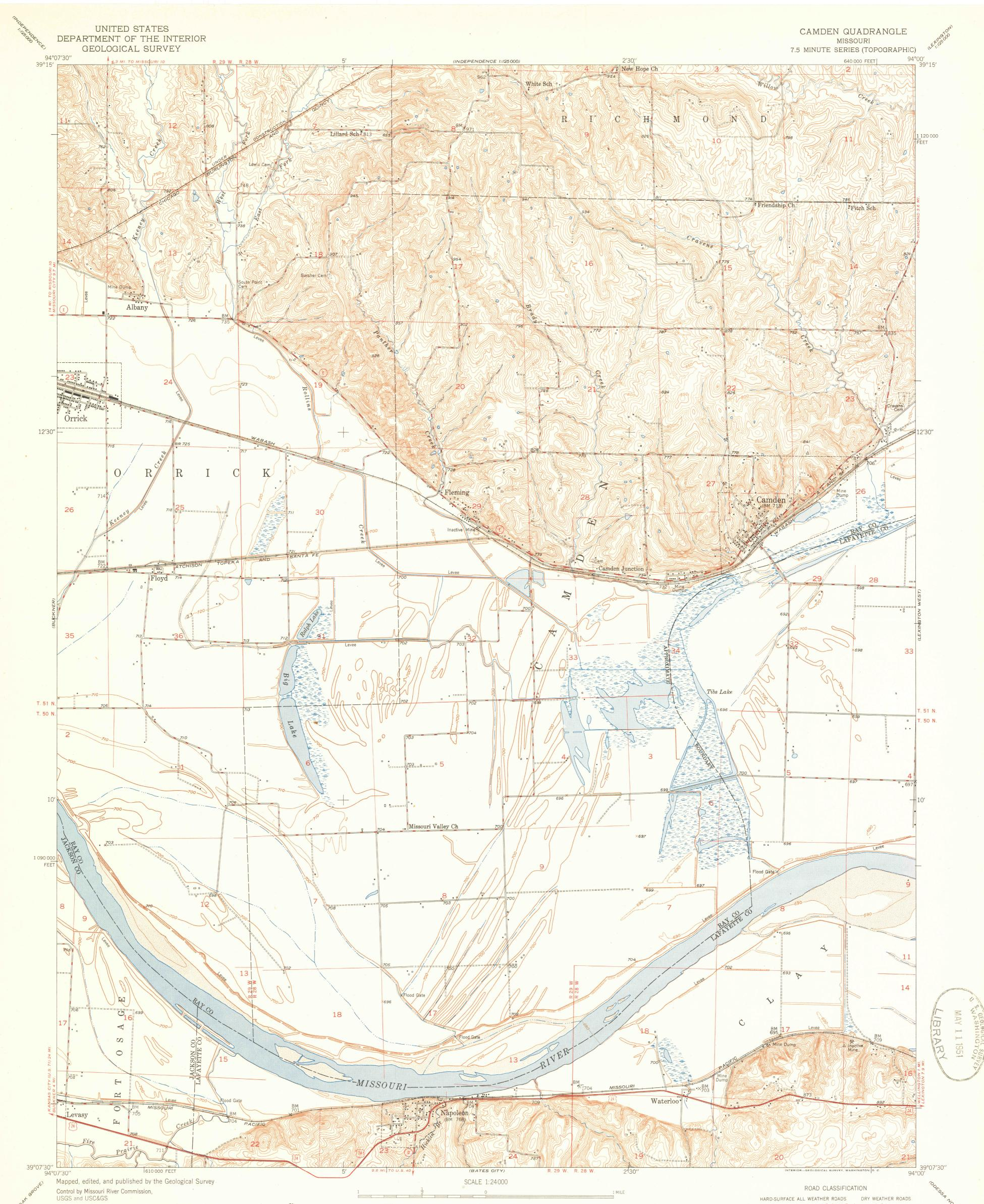
Topography by multiplex methods from aerial photographs taken 1948, and by plane-table surveys 1950 Field check 1950
