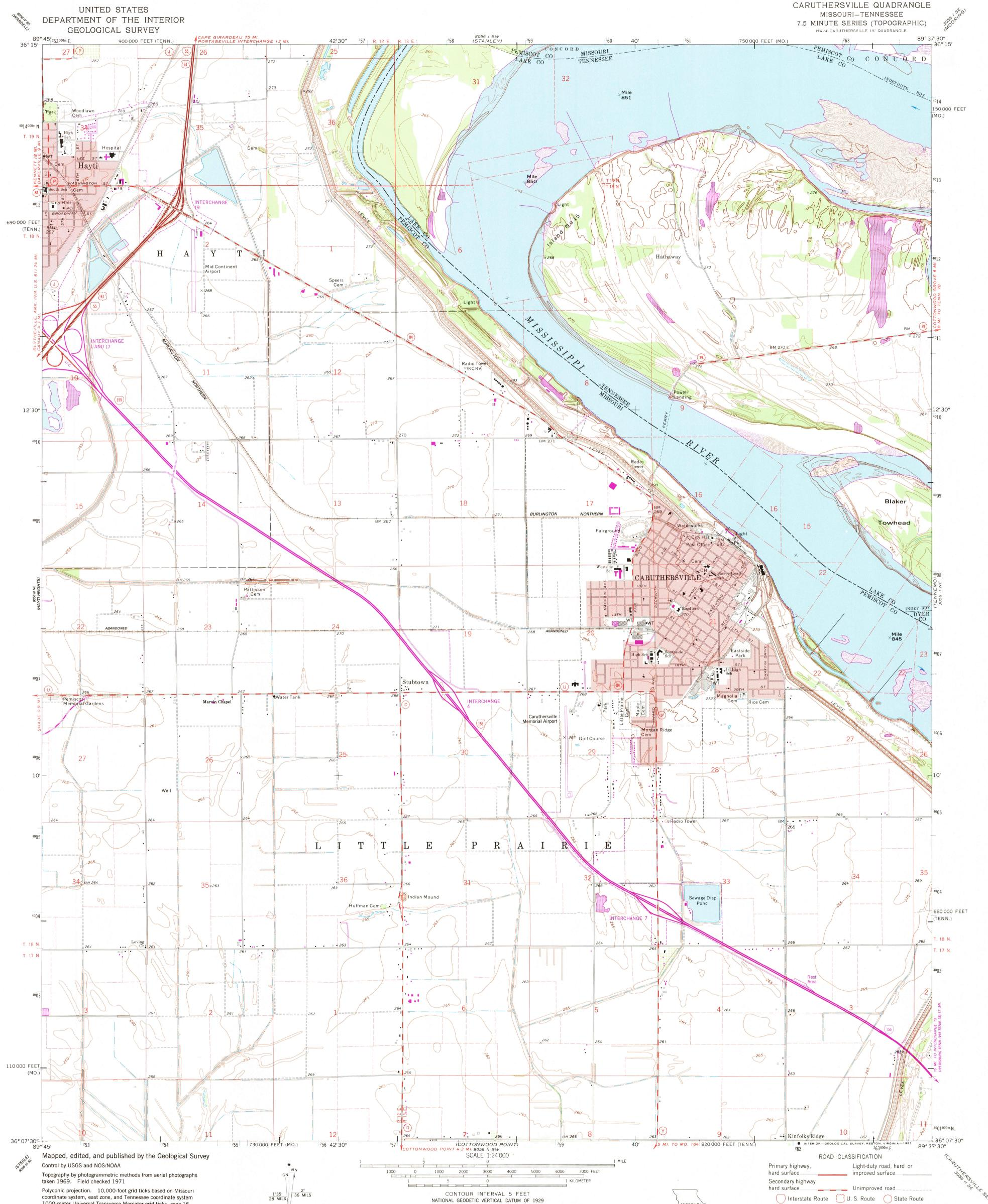
1000-meter Universal Transverse Mercator grid ticks, zone 16, shown in blue. 1927 North American Datum To place on the predicted North American Datum 1983 move the projection lines 5 meters south and 7 meters east as shown by dashed corner ticks Red tint indicates areas in which only landmark buildings are shown
