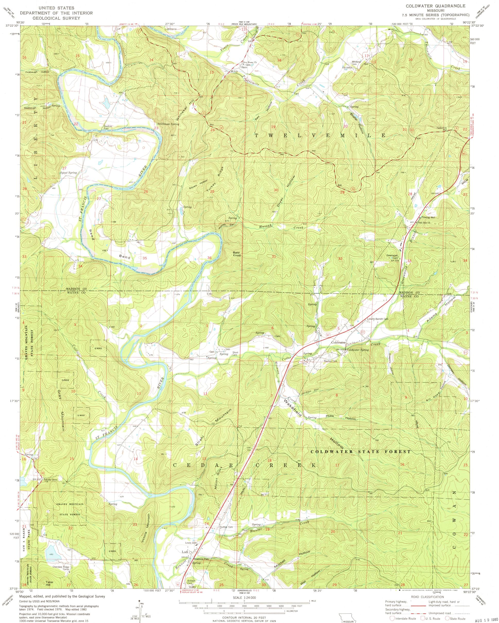
1000-meter Universal Transverse Mercator grid, zone 15 1927 North American Datum To place on the predicted North American Datum 1983 move the projection lines 3 meters south and 9 meters east as shown by dashed corner ticks
