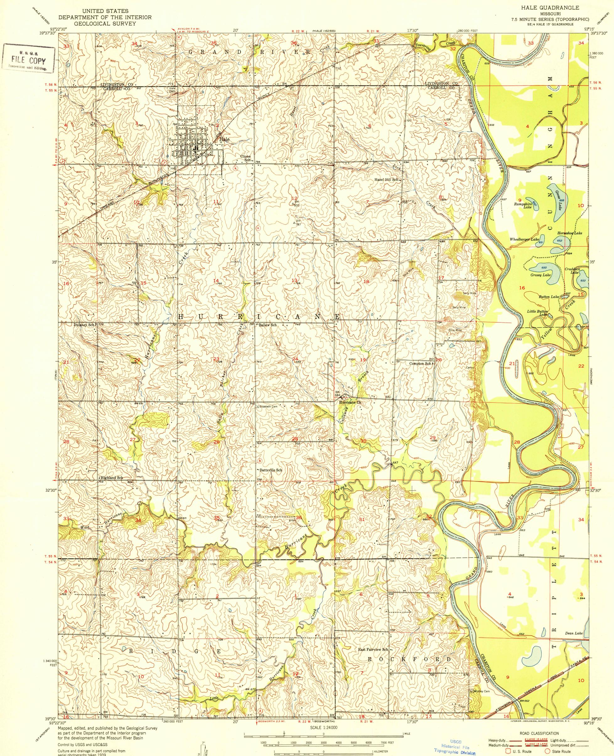
aerial photographs taken 1939 Topography by plane-table methods 1950 Polyconic projection. 1927 North American datum 10,000-foot grid based on Missouri coordinate system, central zone
