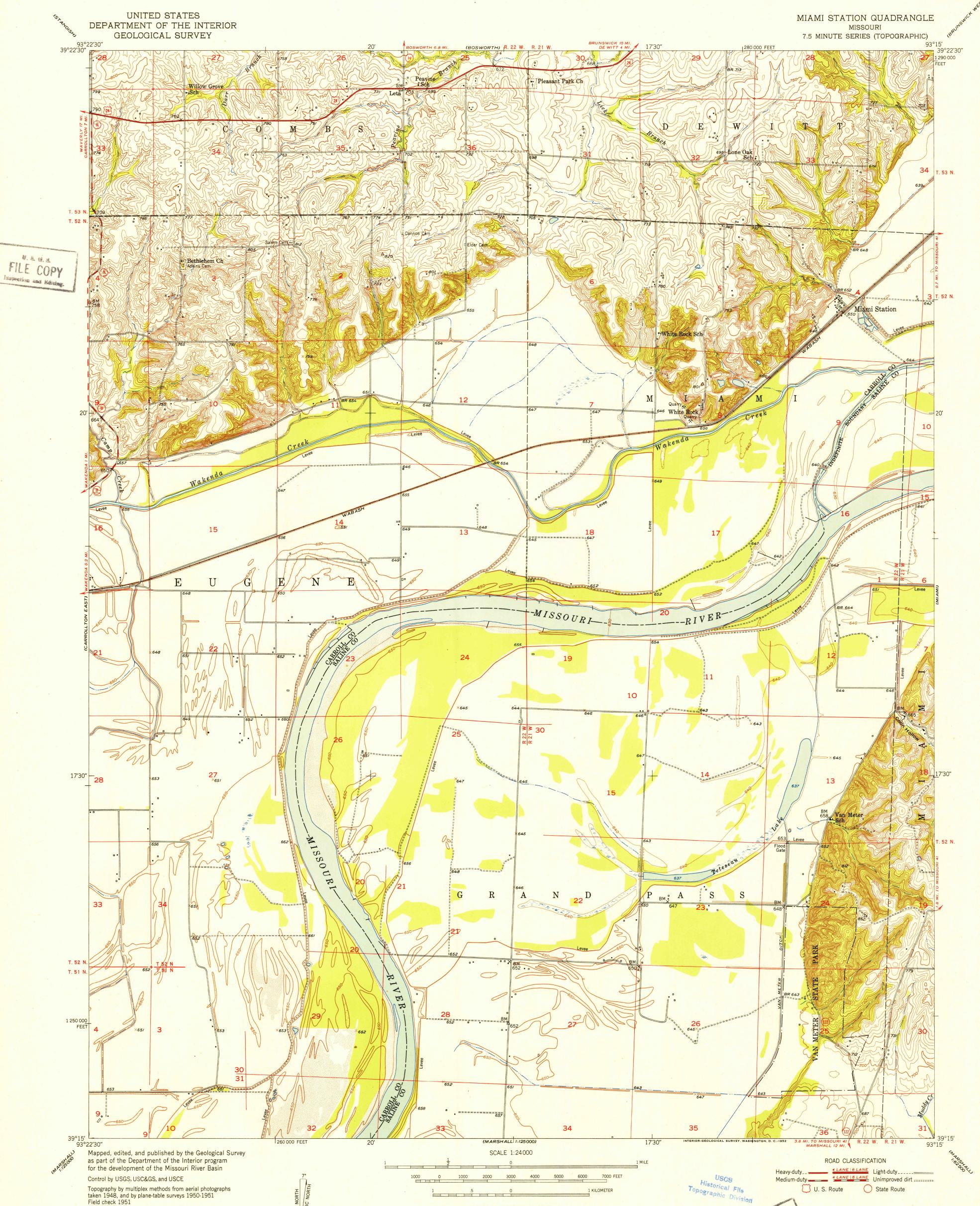
Topography by multiplex methods from aerial photographs taken 1948, and by plane-table surveys 1950-1951 Field check 1951
