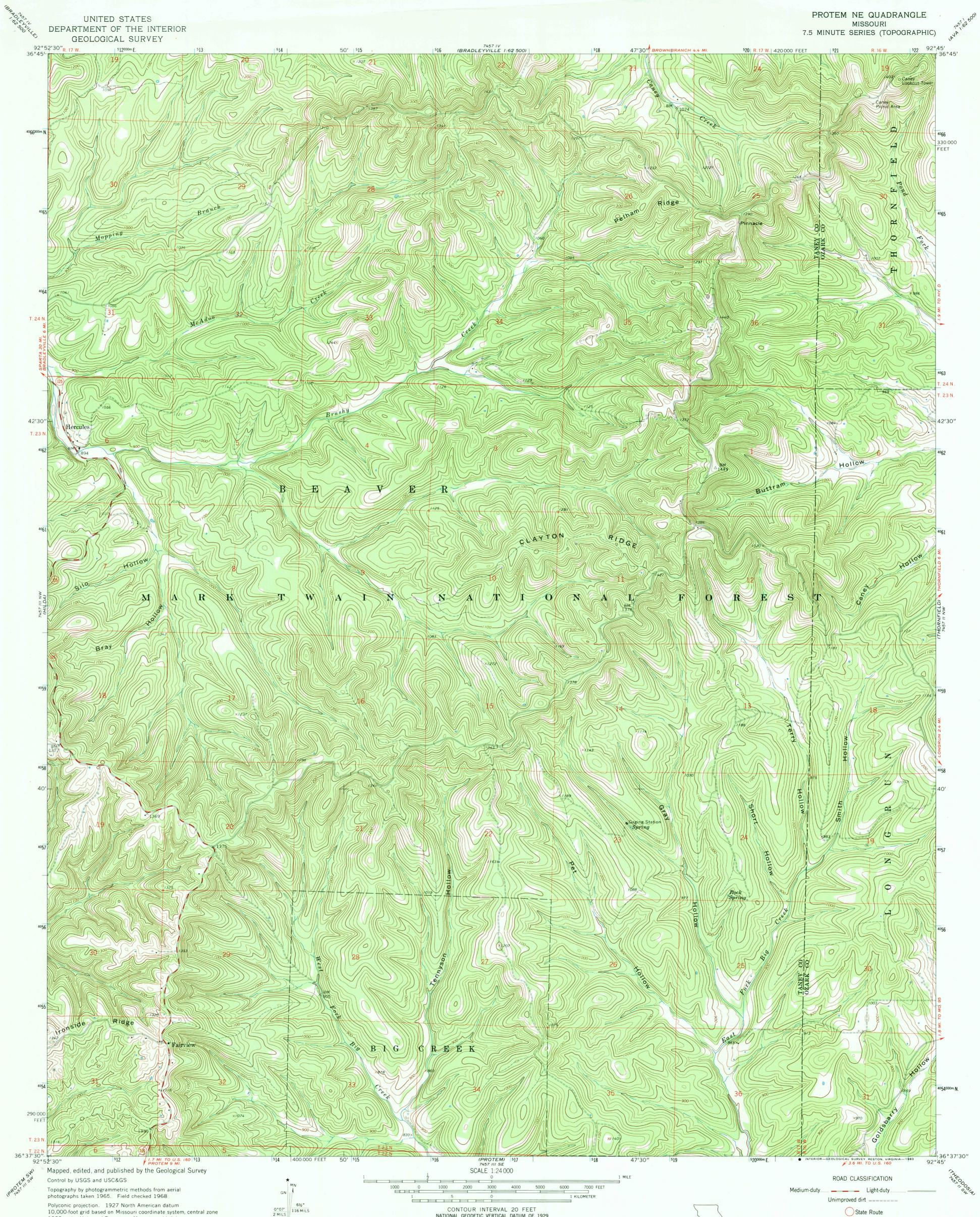
10,000-foot grid based on Missouri coordinate system, central zone 1000-meter Universal Transverse Mercator grid ticks, zone 15, shown in blue To place on the predicted North American Datum 1983, move the projection lines 3 meters south and 15 meters east as shown by dashed corner ticks
