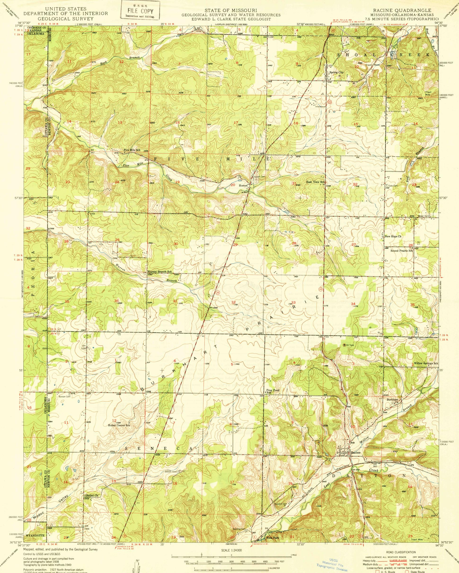
Polyconic projection. 1927 North American datum 10,000-foot grids based on Missouri coordinate system, west zone, Oklahoma coordinate system, north zone, and Kansas coordinate system, south zone
