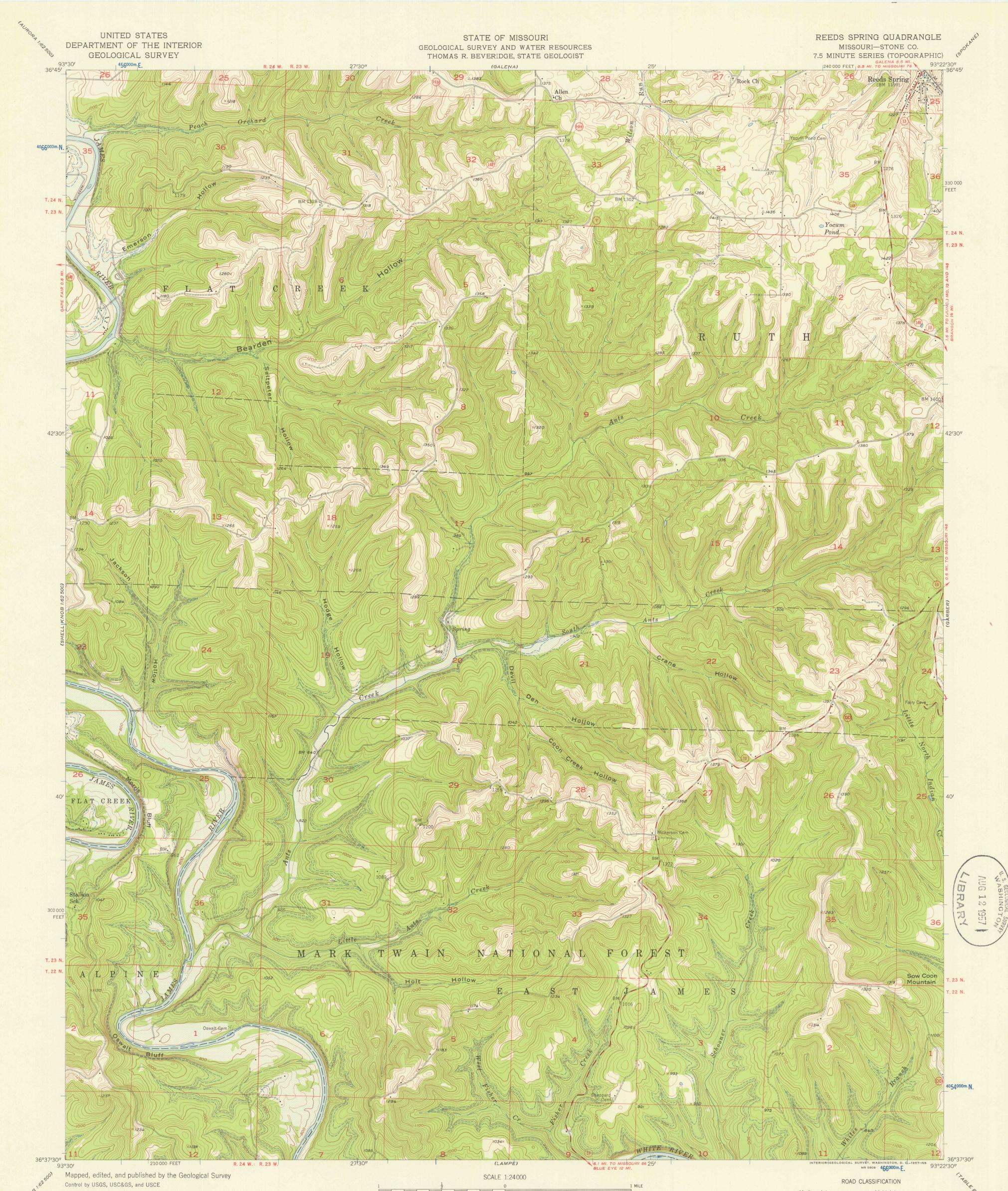
Topography from aerial photographs by multiplex methods Aerial photographs taken 1952. Field check 1956 Polyconic projection. 1927 North American datum 10,000-foot grid based on Missouri coordinate system, central zone 1000-meter Universal Transverse Mercator grid ticks, zone 15, shown in blue
