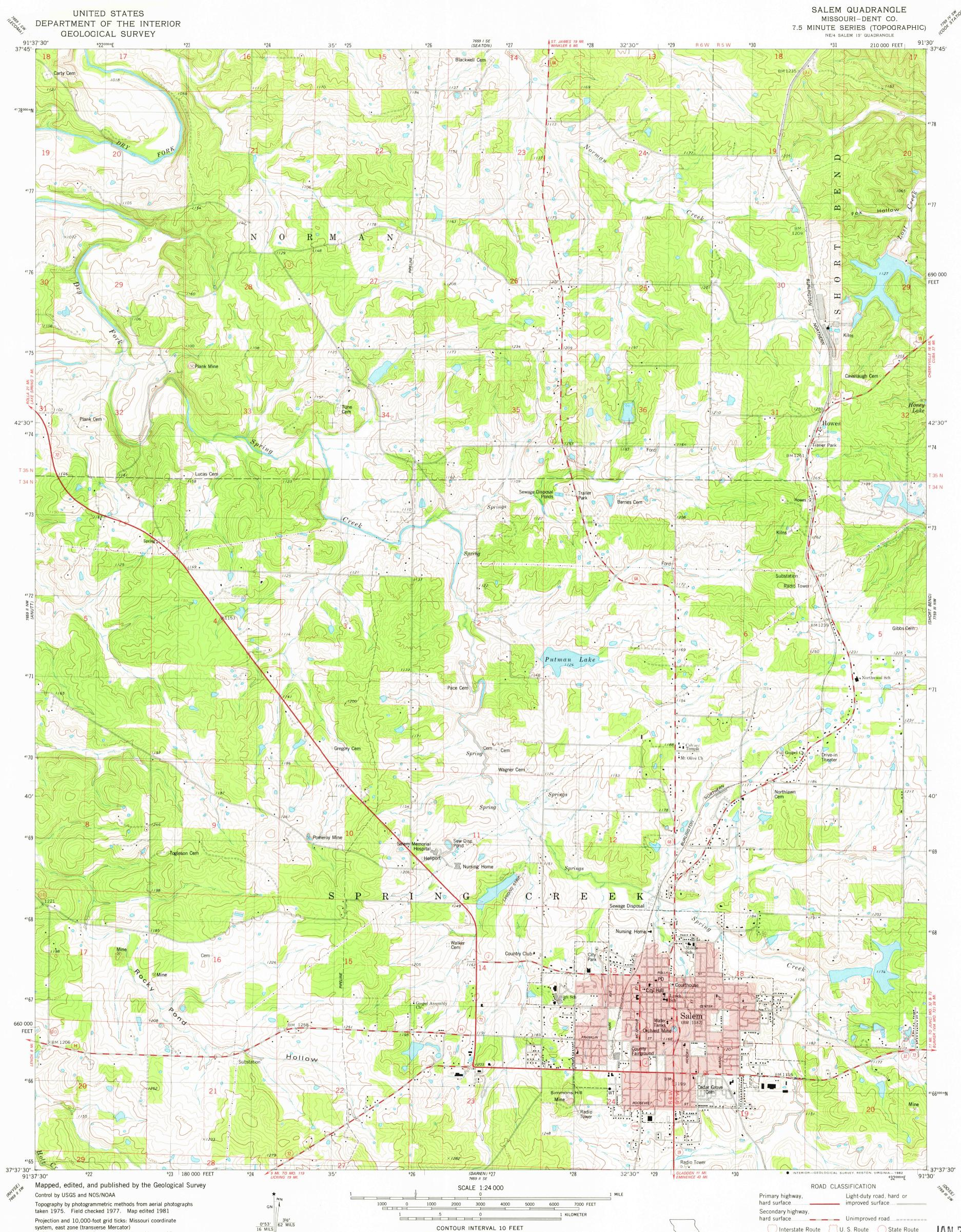
system, east zone (transverse Mercator) 1000-meter Universal Transverse Mercator grid, zone 15 1927 North American Datum To place on the predicted North American Datum 1983 move the projection lines 2 meters south and 12 meters east as shown by dashed corner ticks Red tint indicates area in which only landmark buildings are shown Fine red dashed lines indicate selected fence and field lines where generally visible on aerial photographs. This information is unchecked
