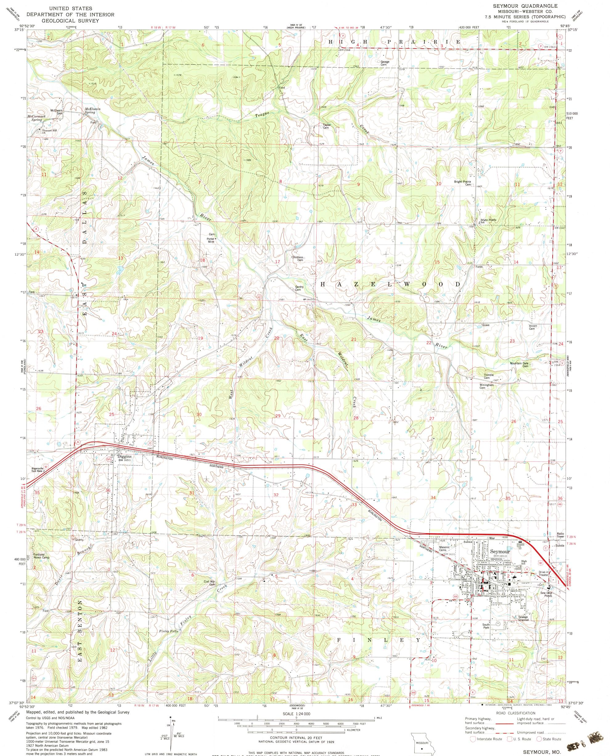
system, central zone (transverse Mercator) 1000-meter Universal Transverse Mercator grid, zone 15 1927 North American Datum To place on the predicted North American Datum 1983 move the projection lines 3 meters south and 15 meters east as shown by dashed corner ticks
