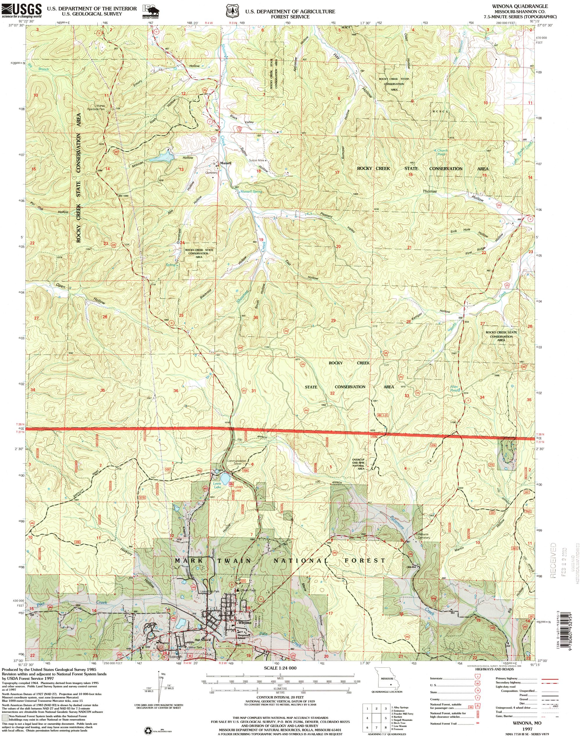
Blue 1000-meter Universal Transverse Mercator ticks, zone 15 North American Datum of 1983 (NAD 83) is shown by dashed corner ticks The values of the shift between NAD 27 and NAD 83 for 7.5-minute intersections are obtainable from National Geodetic Survey NADCON software
