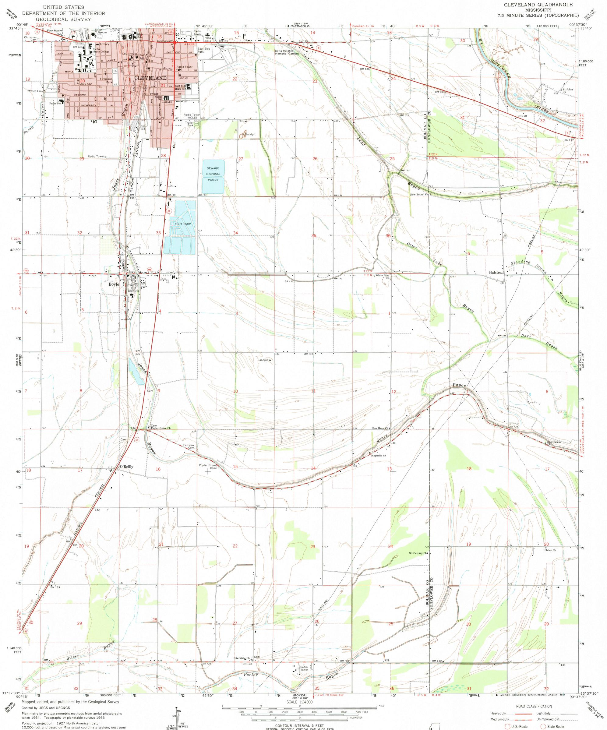
10,000-foot grid based on Mississippi coordinate system, west zone 1000-meter Universal Transverse Mercator grid ticks, zone 15, shown in blue To place on the predicted North American Datum 1983, move the projection lines 10 meters south and 10 meters east as shown by dashed corner ticks
