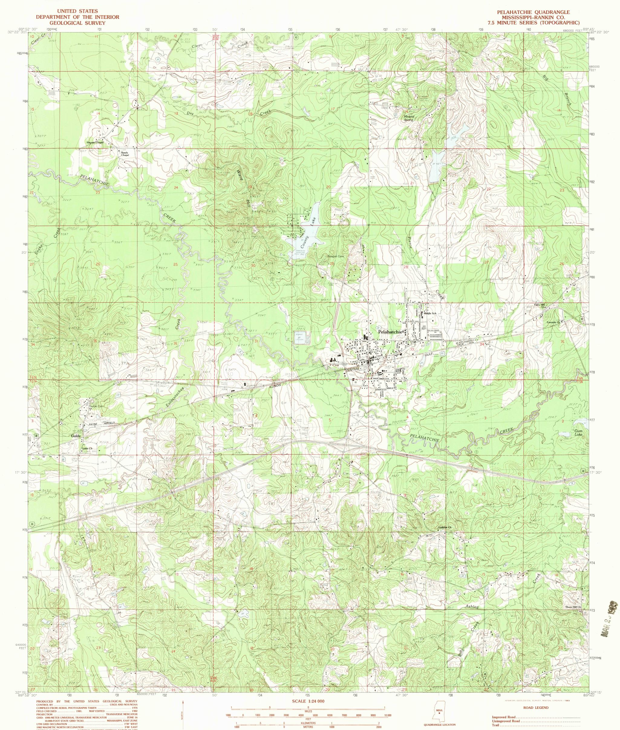
VERTICAL DATUM ...... NATIONAL GEODETIC VERTICAL DATUM OF 1929 HORIZONTAL DATUM ..... 1927 NORTH AMERICAN DATUM To place on the predicted North American Datum of 1983 move the projection lines as shown by dashed corner ticks (13 meters south and 7 meters east) There may be private inholdings within the boundaries of any Federal and State reservations shown on this map
