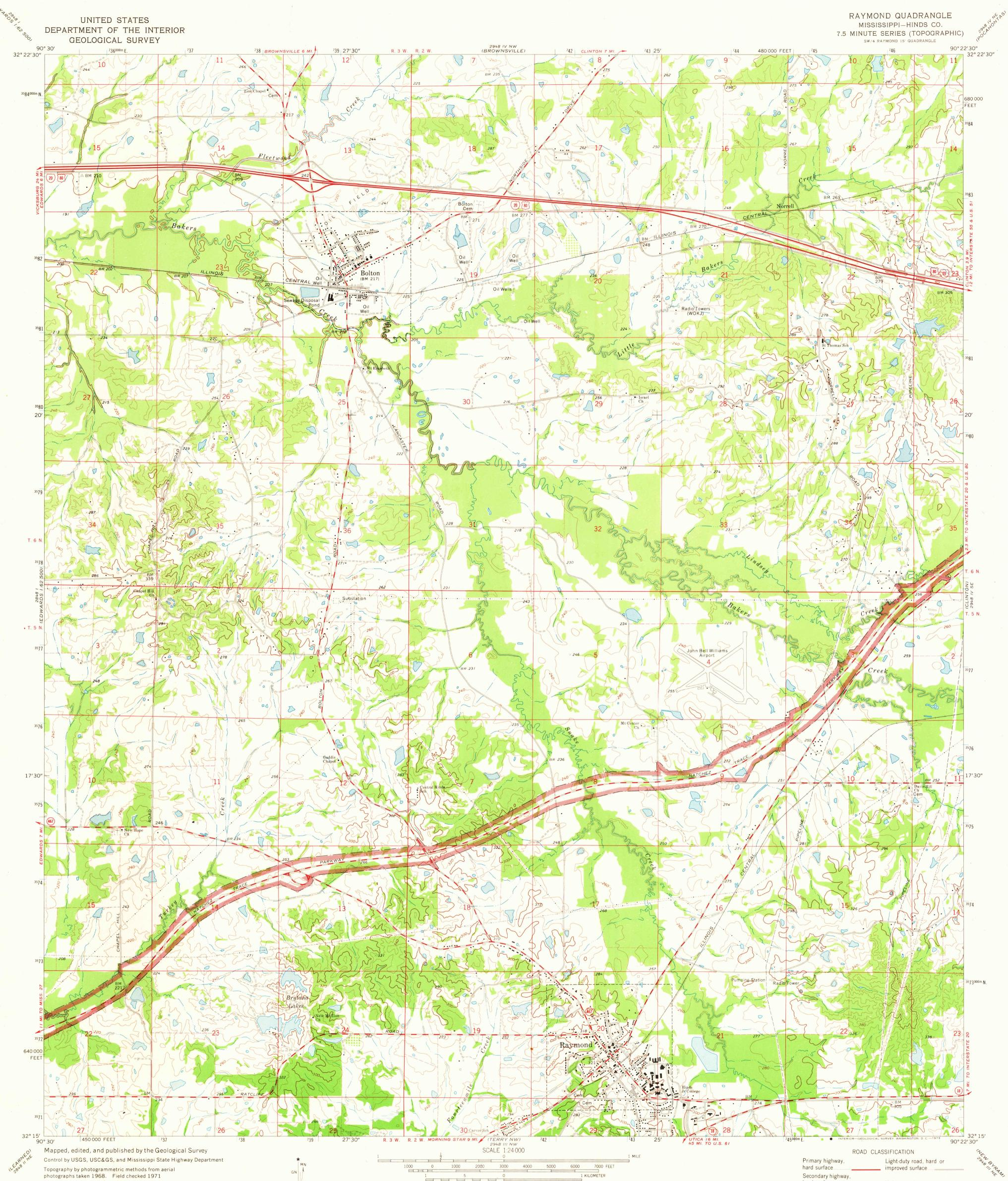
Polyconic projection. 1927 North American datum 10,000-foot grid based on Mississippi coordinate system, west zone 1000-meter Universal Transverse Mercator grid ticks, zone 15, shown in blue
