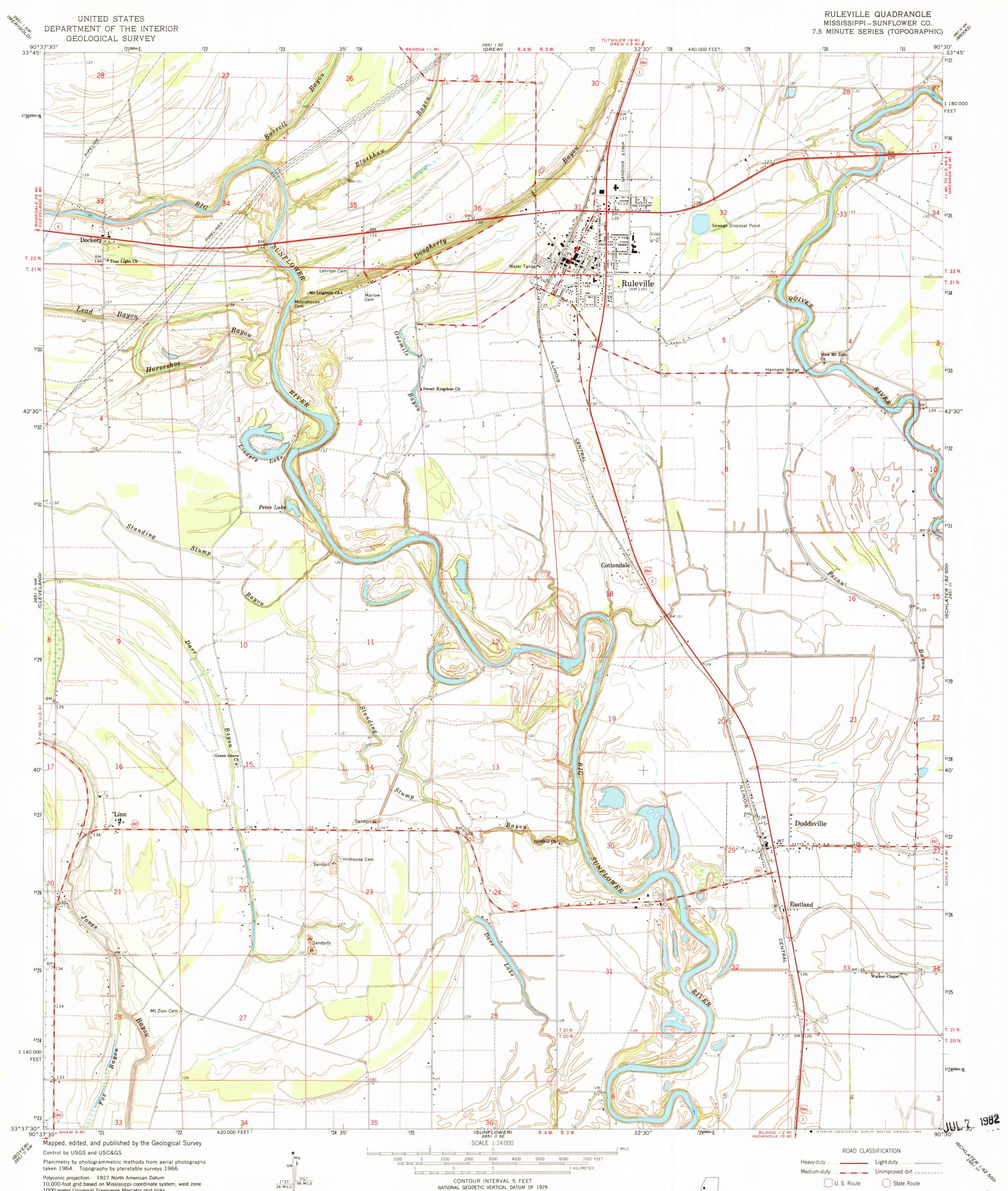
Polyconic projection. 1927 North American Datum 10,000-foot grid based on Mississippi coordinate system, west zone 1000-meter Universal Transverse Mercator grid ticks, zone 15, shown in blue To place on the predicted North American Datum 1983 move the projection lines 10 meters south and 9 meters east as shown by dashed corner ticks
