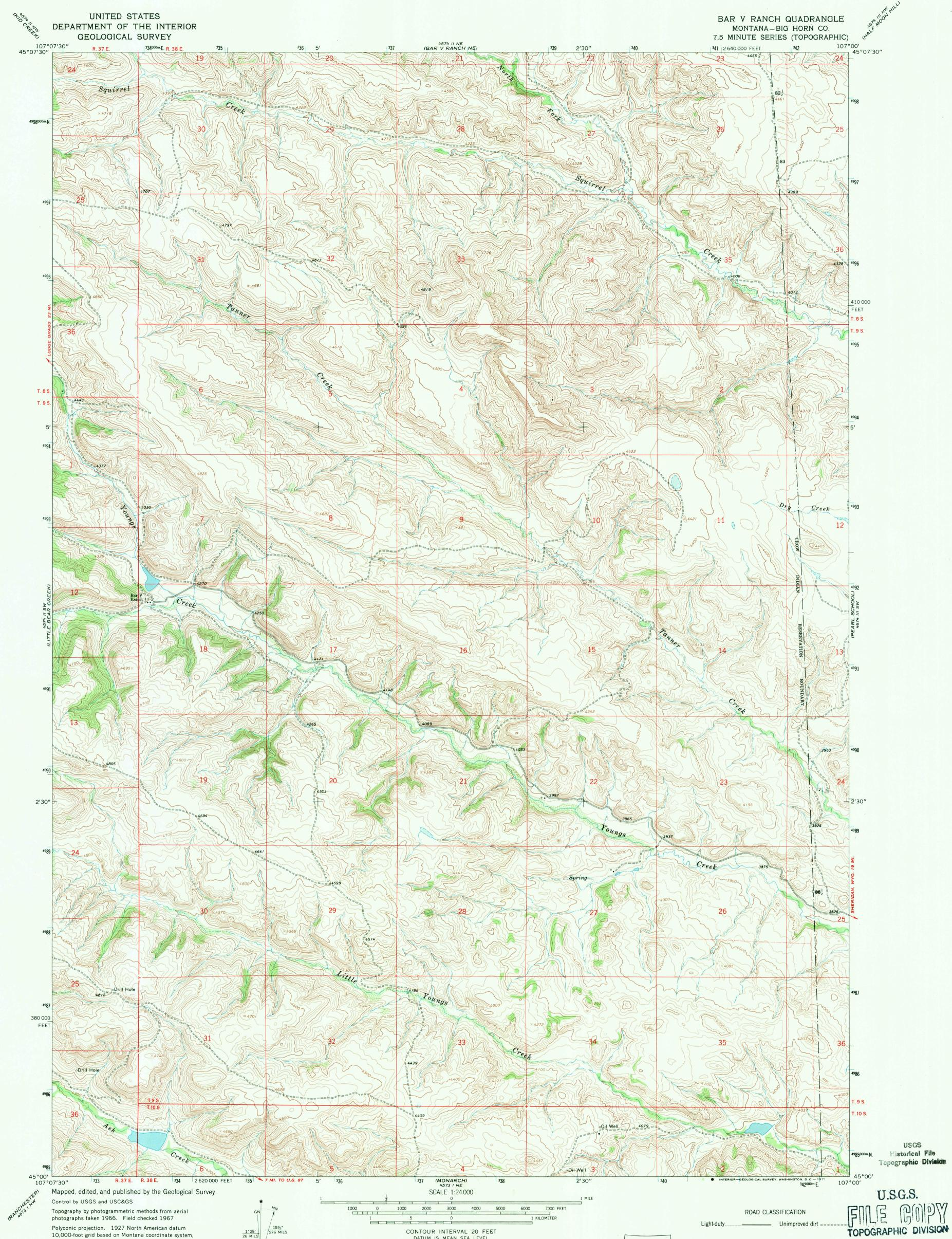
Polyconic projection. 1927 North American datum 1°28' 276 MILS 10,000-foot grid based on Montana coordinate system, south zone 1000-meter Universal Transverse Mercator grid ticks, zone 13, shown in blue UTM GRID AND 1967 MAGNETIC NORTH DECLINATION AT CENTER OF SHEET Fine red dashed lines indicate selected fence lines
