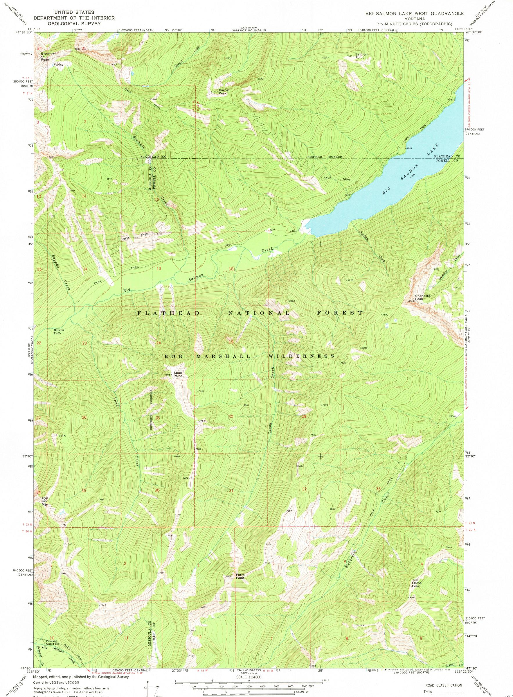
Polyconic projection. 1927 North American datum 10,000-foot grids based on Montana coordinate system, central and north zones 1000-meter Universal Transverse Mercator grid ticks, zone 12, shown in blue UTM GRID AND 1970 MAGNETIC NORTH DECLINATION AT CENTER OF SHEET Where omitted, land lines have not been established To place on the predicted North American Datum 1983 move the projection lines 11 meters north and 68 meters east as shown by dashed corner ticks
