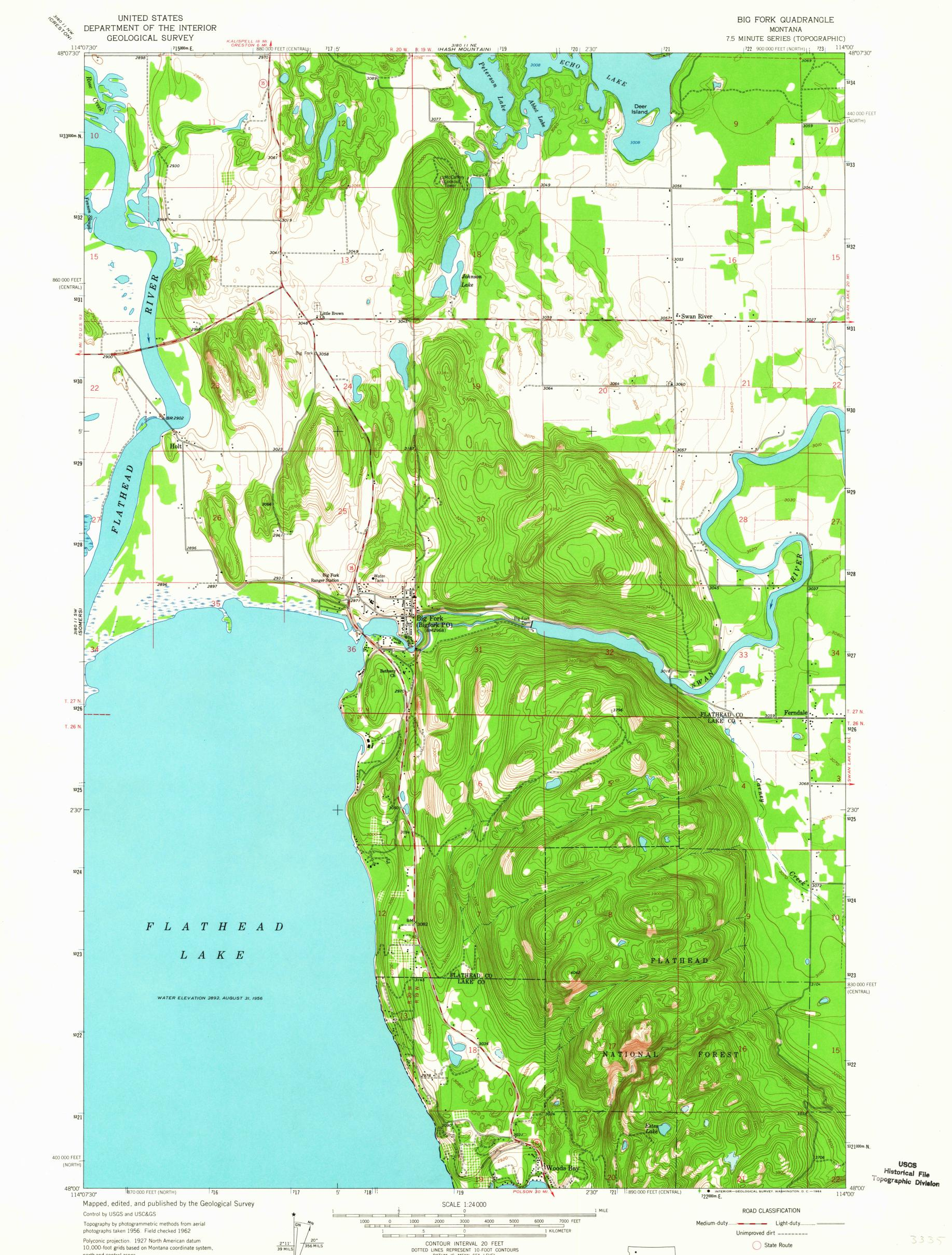
Polyconic projection. 1927 North American datum 10,000 foot grids based on Montana coordinate system, north and central zones 1000-meter Universal Transverse Mercator grid ticks, zone 11, shown in blue Fine red dashed lines indicate selected fence lines
