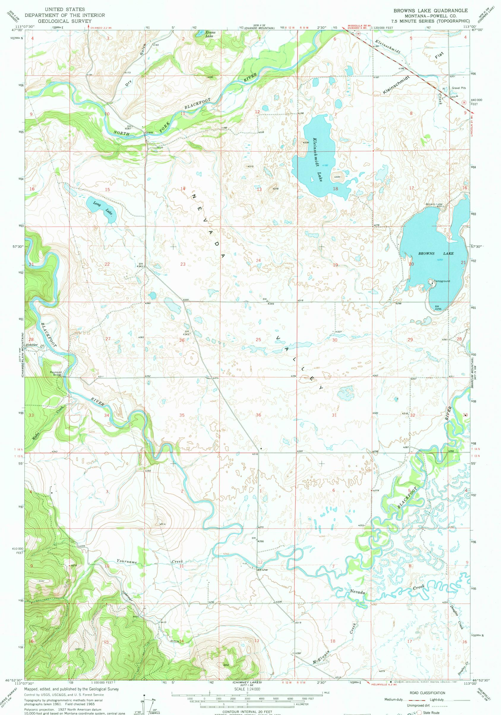
Polyconic projection. 1927 North American datum 1°30' 27 MILS 10,000-foot grid based on Montana coordinate system, central zone 1000-meter Universal Transverse Mercator grid ticks, zone 12, shown in blue
