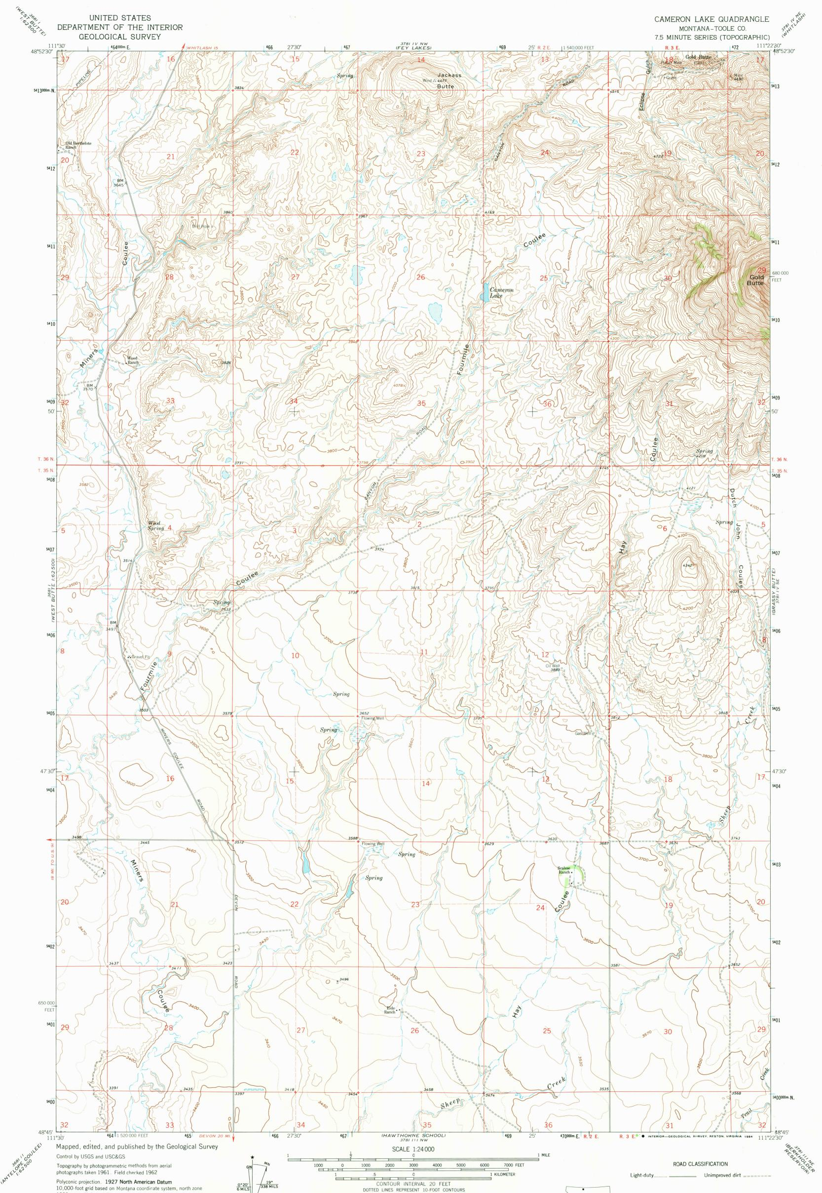
Polyconic projection. 1927 North American Datum 10,000-foot grid based on Montana coordinate system, north zone 1000-meter Universal Transverse Mercator grid ticks, zone 12, shown in blue
