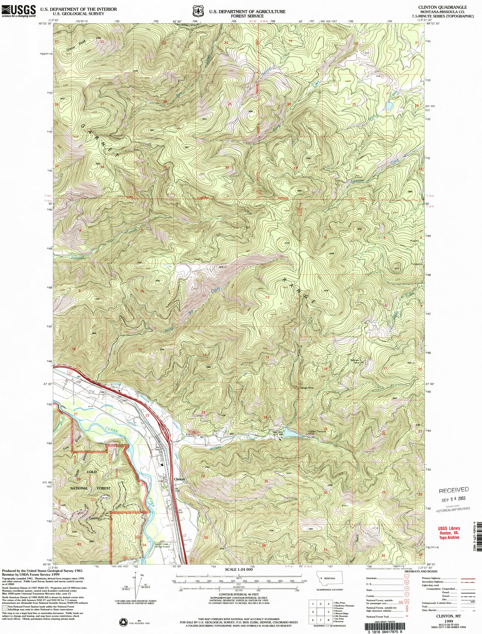
Montana coordinate system, central zone (Lambert conformal conic) Blue 1000-meter Universal Transverse Mercator ticks, zone 12
