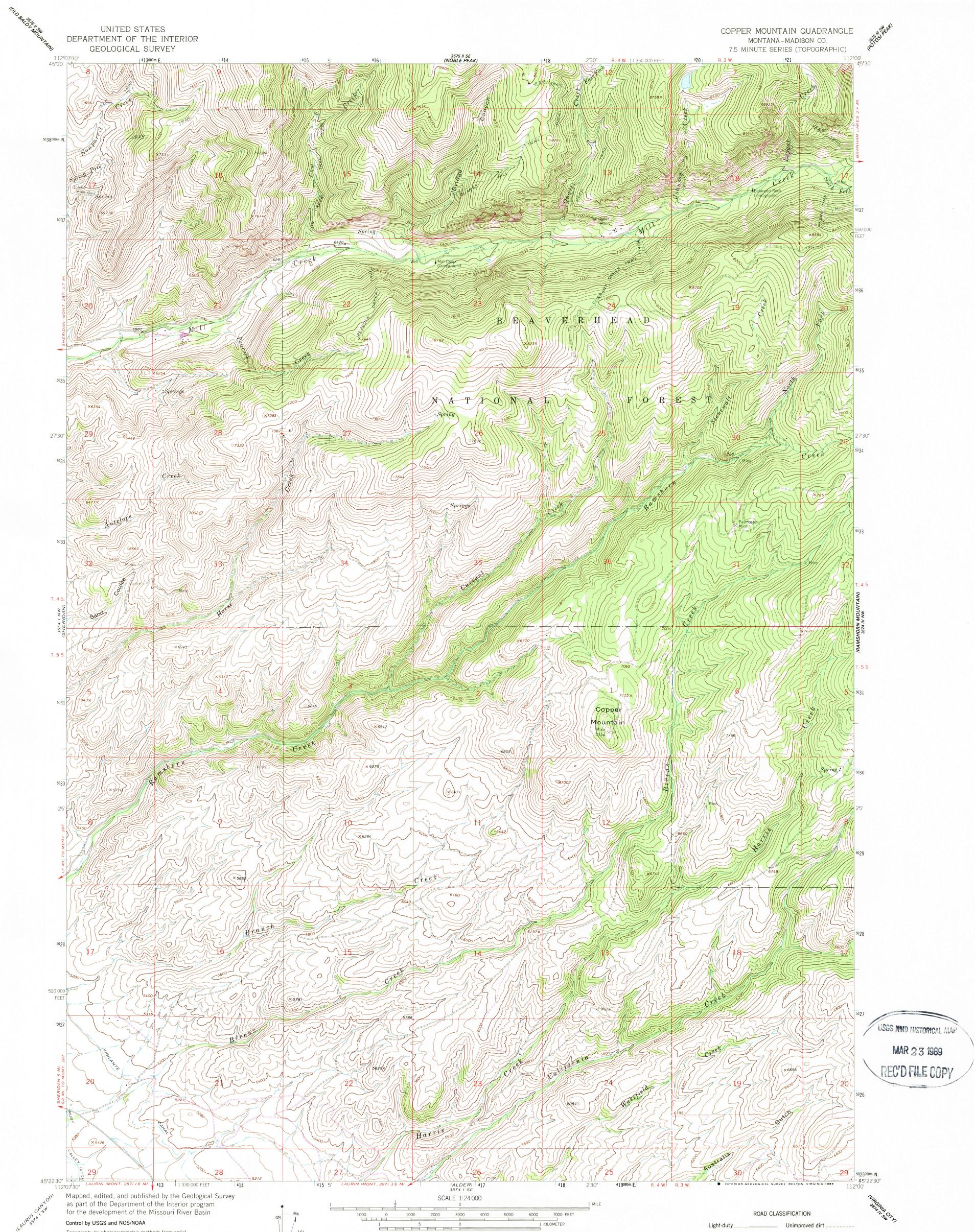
Topography by photogrammetric methods from aerial photographs taken 1961. Field checked 1963 Polyconic projection. **1927 North American Datum** 10,000-foot grid based on Montana coordinate system, south zone 1000-meter Universal Transverse Mercator grid ticks, zone 12, shown in blue Fine red dashed lines indicate selected fence lines To place on the predicted North American Datum 1983 move the projection lines 11 meters north
