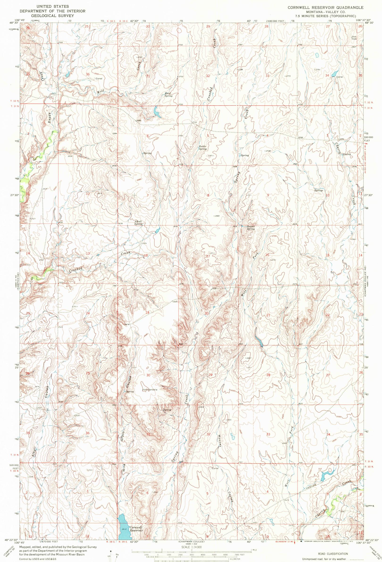
Topography by photogrammetric methods from aerial photographs taken 1967. Field checked 1969 Polyconic projection. 1927 North American datum
