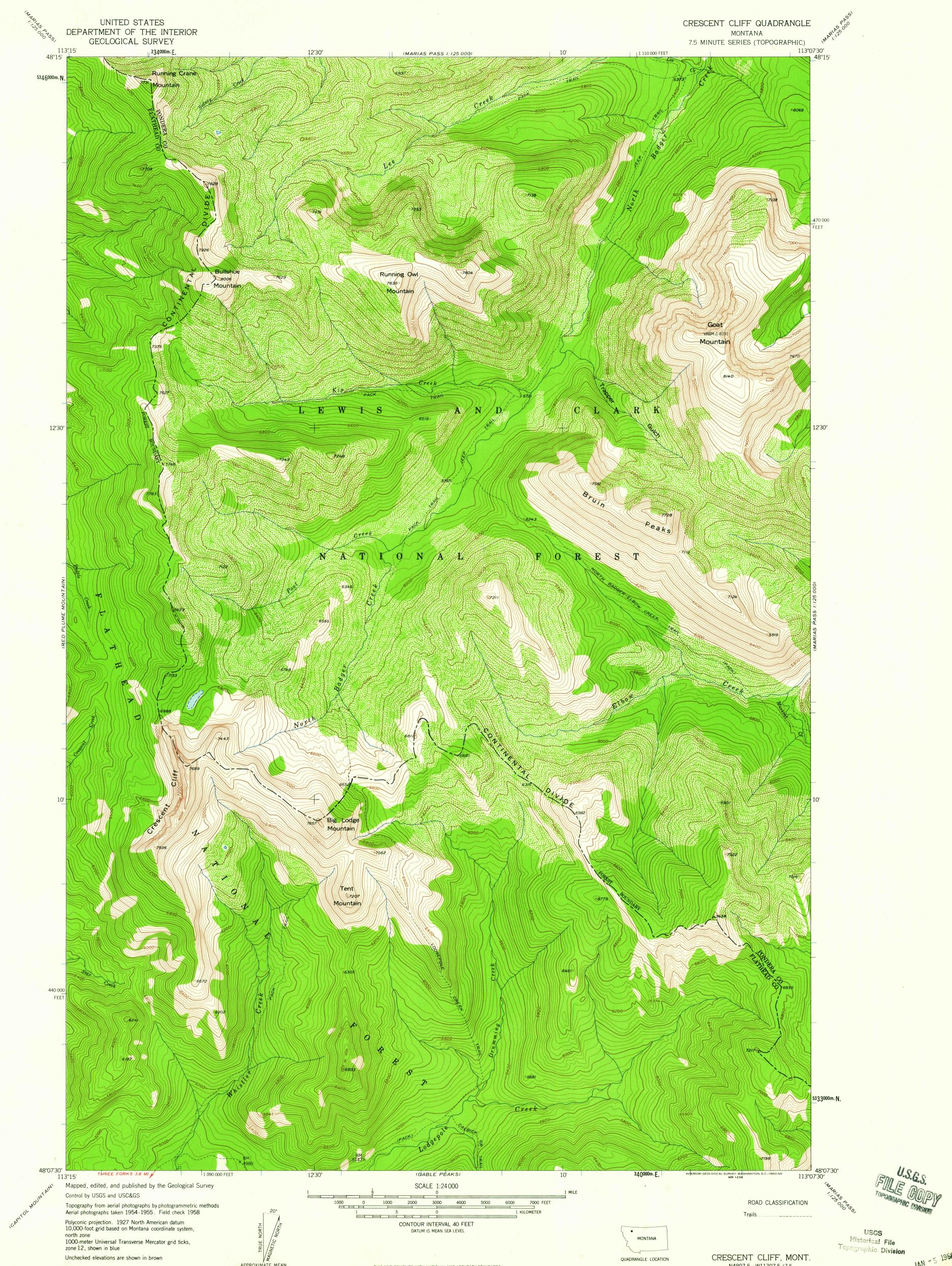
Polyconic projection. 1927 North American datum 10,000-foot grid based on Montana coordinate system, north zone 1000-meter Universal Transverse Mercator grid ticks, zone 12, shown in blue Unchecked elevations are shown in brown
