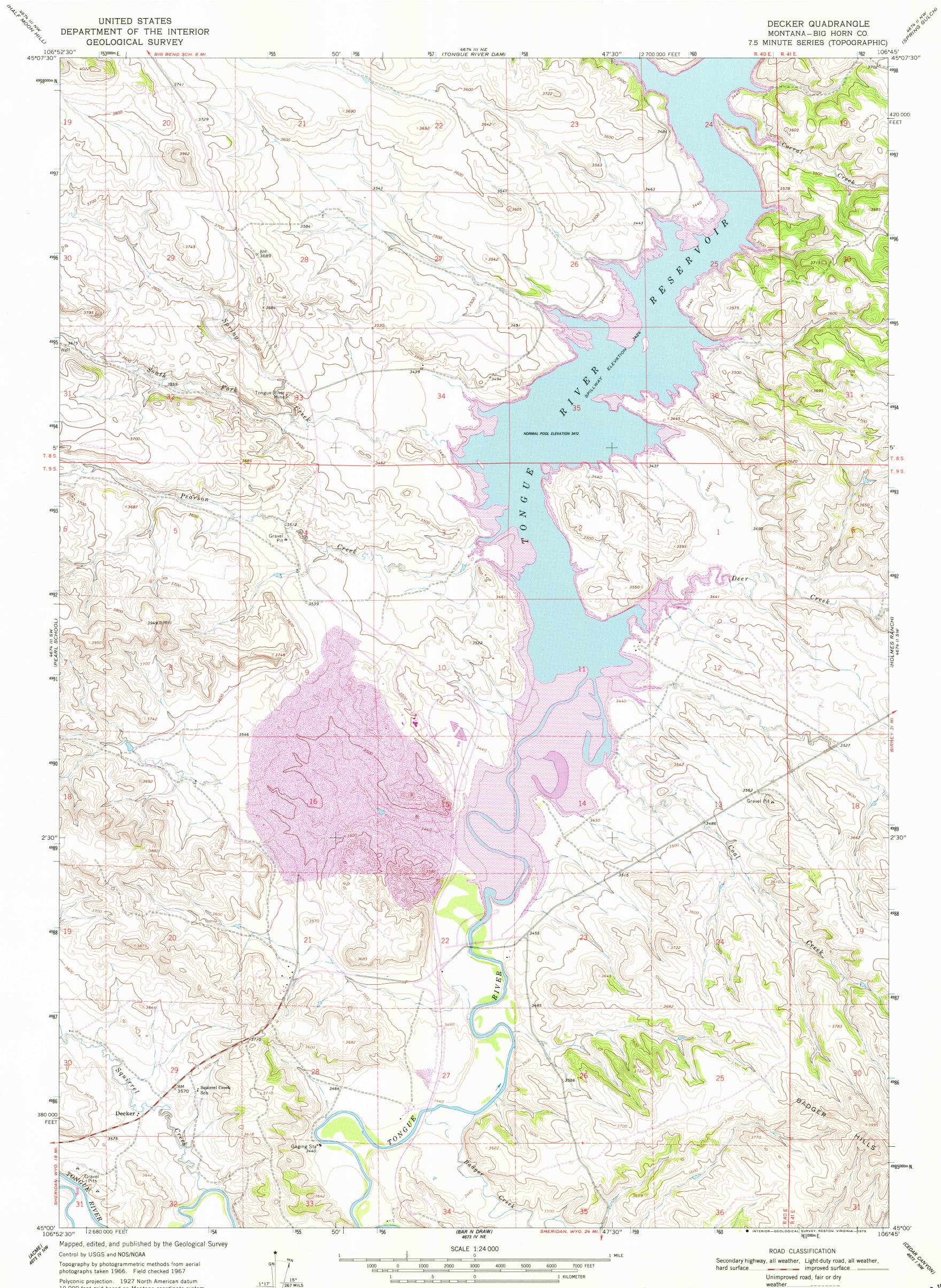
10,000-foot grid based on Montana coordinate system, 23 MILS south zone 1000-meter Universal Transverse Mercator grid ticks, zone 13, shown in blue Fine red dashed lines indicate selected fence lines
